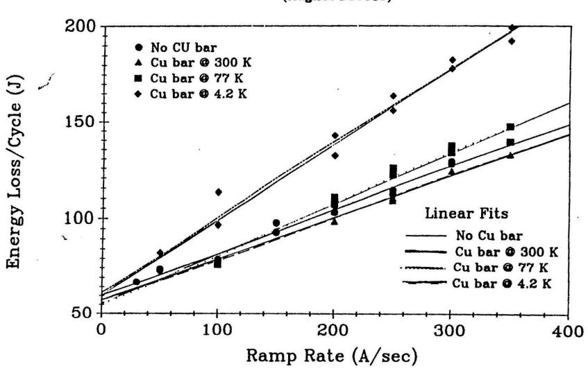
• BIPOLAR STANDARD RAMP: RAMP RATE STUDY WITH dI/dt = 60, 100, 150, 200, 250, 300 A/sec; SYMMETRIC RAMP WITH 5 SECOND DWELLS AT I<sub>MIN</sub>, I<sub>MAX</sub>, AND AT I = 0
