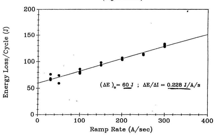
Energy Loss as a Function of Ramp Rate (Magnet DS0315)
