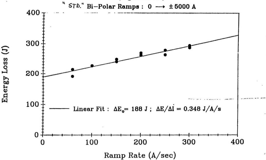
Energy Loss as a Function of Ramp Rate
