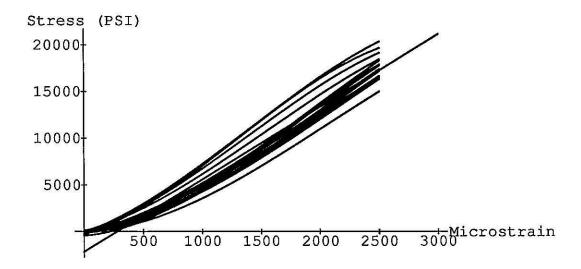
FNL gages calibrated at FNL at about  $300^{\circ}$ K. The line shown is the best linear fit to these curves over the range of 200 to 2500 microstrain. It has the form -2162+7.76x.
