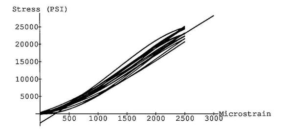
FNL gages calibrated at FNL at about  $4.2^{\circ}$ K. The line shown is the best linear fit to these curves over the range of 200 to 2500 microstrain. It has the form -2681+10.3x.
