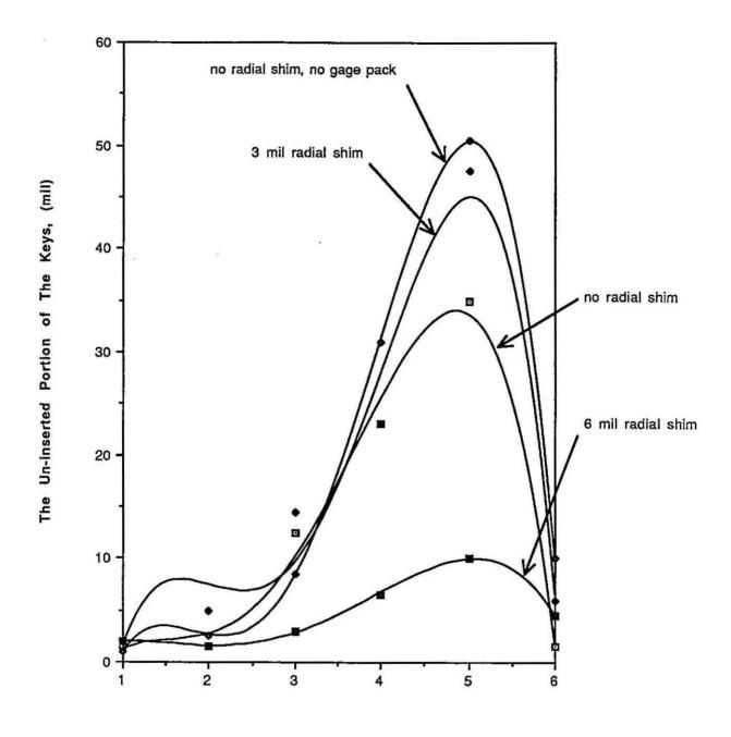
Figure 10: Collaring with a 7 mil vertical shim, at 9400 hydraulic psi, checking for the effects of different radial shims & transducer packs.
