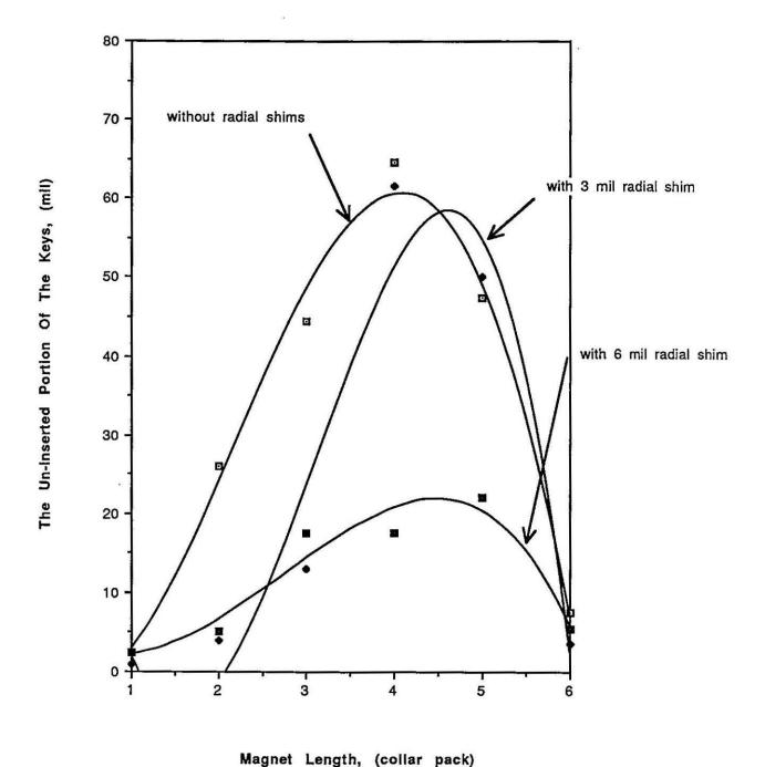
Figure 5: Comparing the effects of different radial shims
