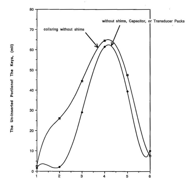
Figure 4: Collaring without radial shims, at 9400 hydraulic psi, checking for the effects of removing the transducer & capacitor packs.
