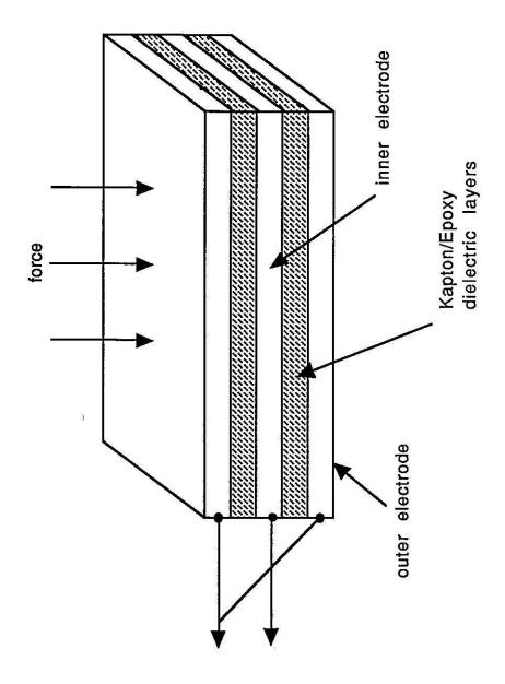
Figure 20: Kapton-Epoxy gage
