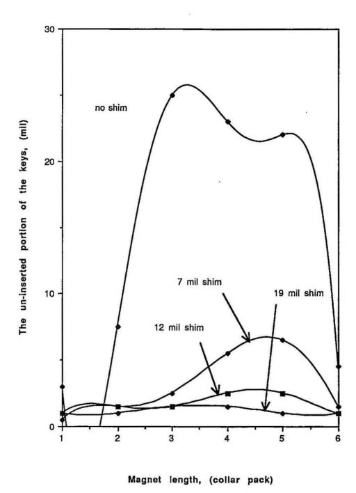
Figure 17: Collaring at the middle of the press with various vertical shims
