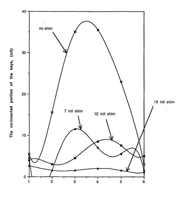
Figure 16: Collaring at the end of the press, with various vertical shims
