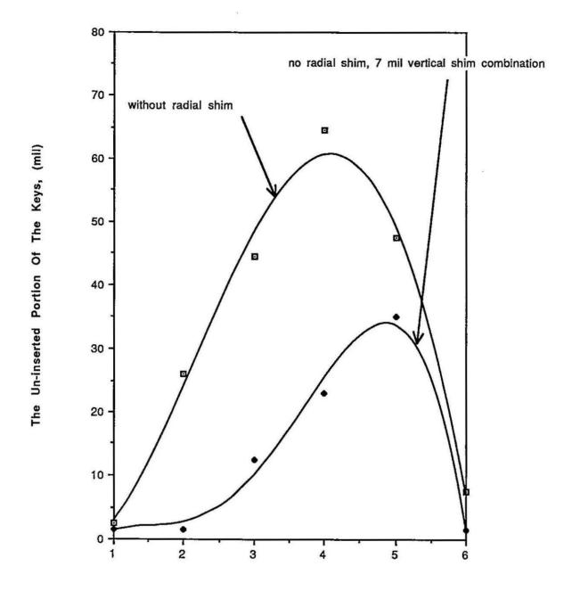
Figure 7: Collaring without radial shims, checking for the effects of a 7 mil vertical shim
