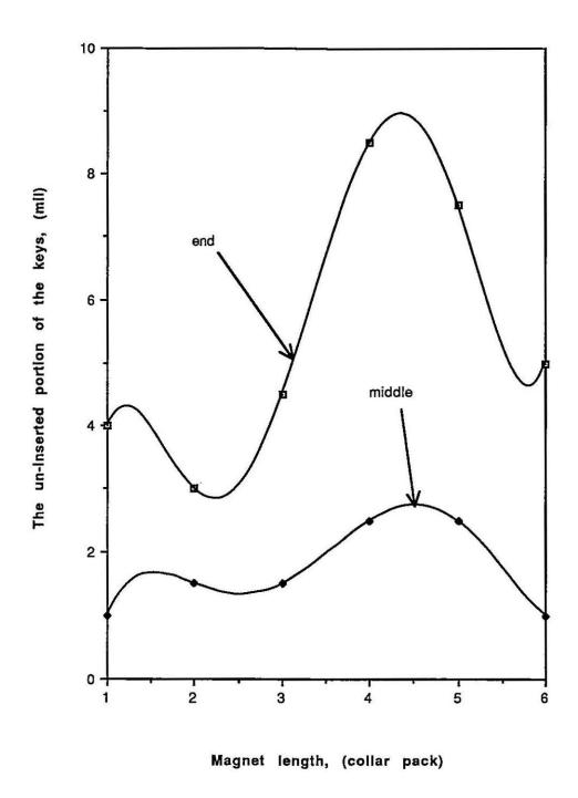
Figure 14: Collaring at the end & middle of the press with 12 mil vertical shim
