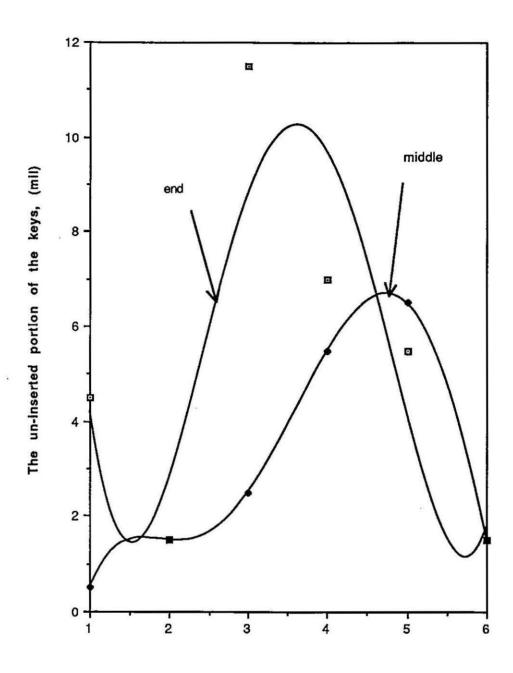
Figure 13: Collaring at the end & middle of the press with 7 mil vertical shim
