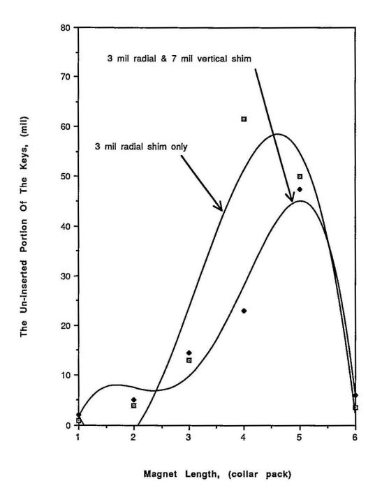
Figure 8: Collaring with 3 mil radial shims, at 9400 hydraulic psi, also checking for the effects of a 7 mil vertical shim.
