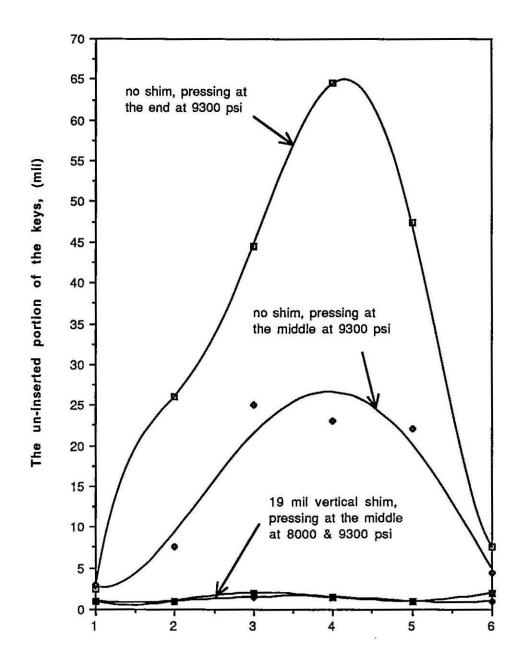
Figure 18: Collaring at different press positions & pressures
