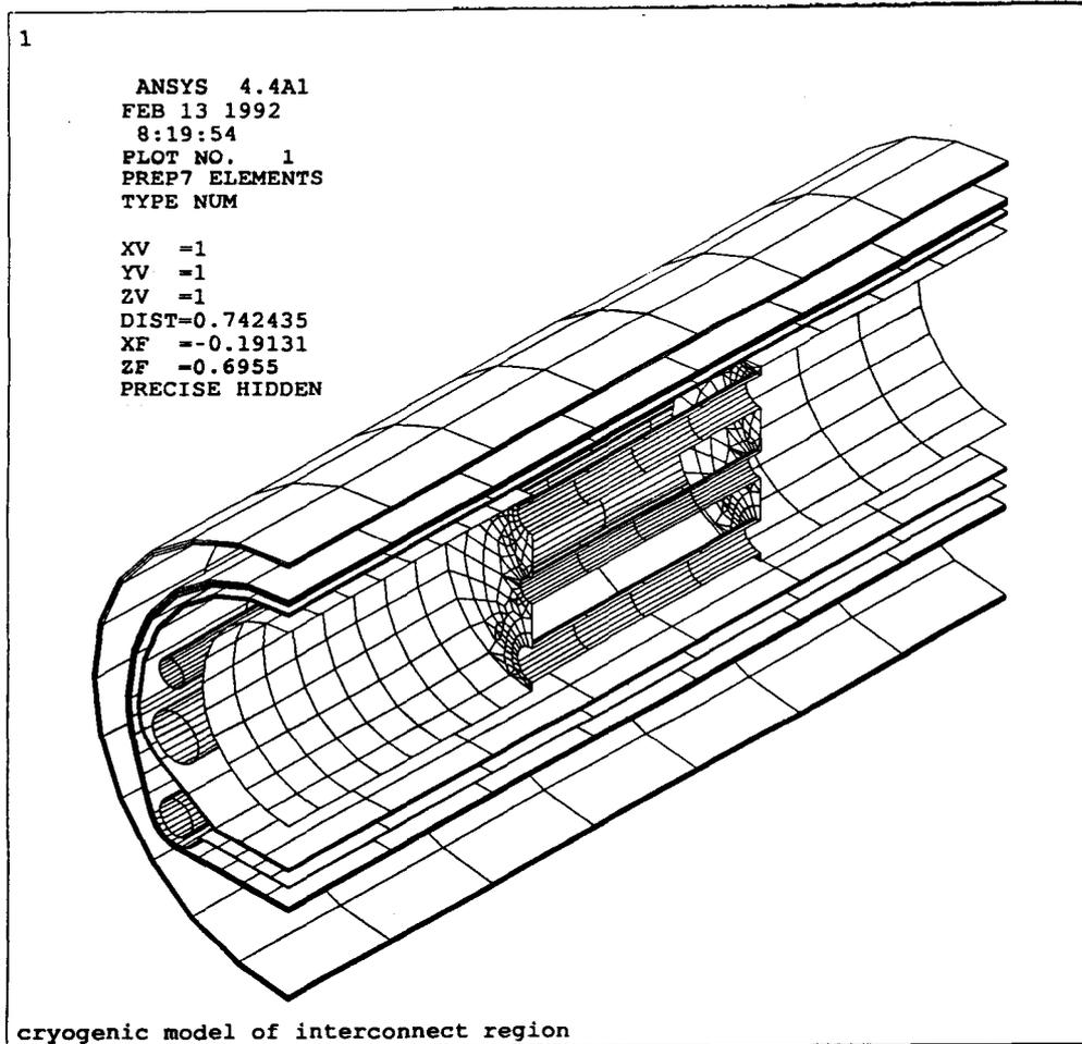
Figure 3. Finite Element Mesh of the Interconnect Region.
