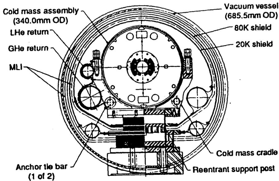
Figure 1. 50-mm Collider Dipole Cryostat Cross Section.
