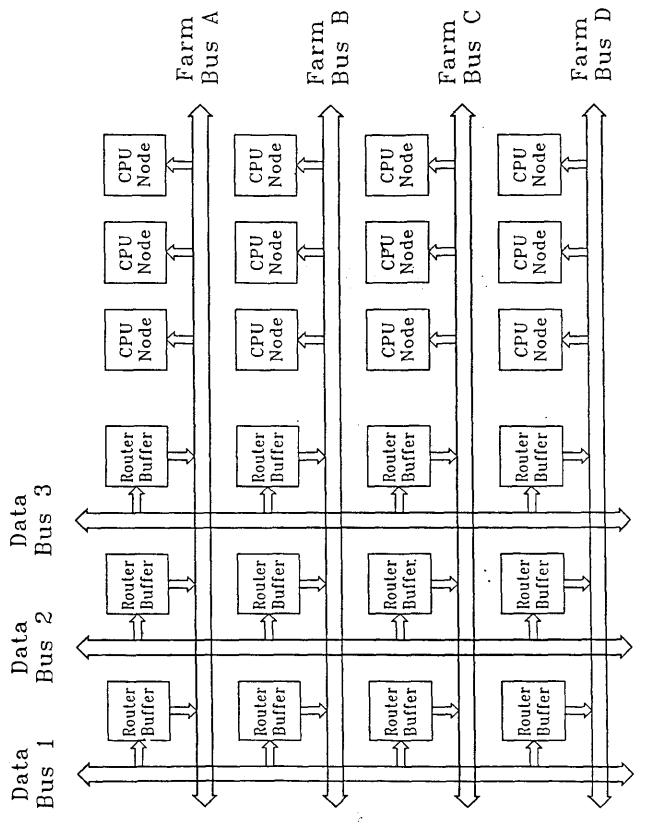
Fig. 3. Event Builder Architecture Based on Dual-Port Memories.
