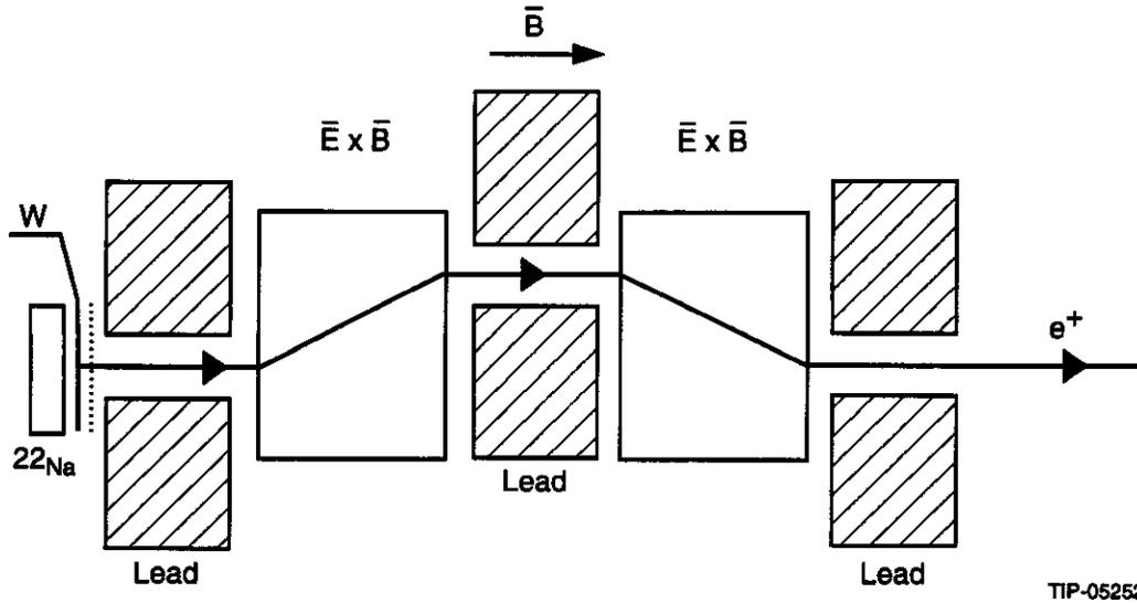
Figure 1. Main components of a magnetically guided low energy positron beam.
