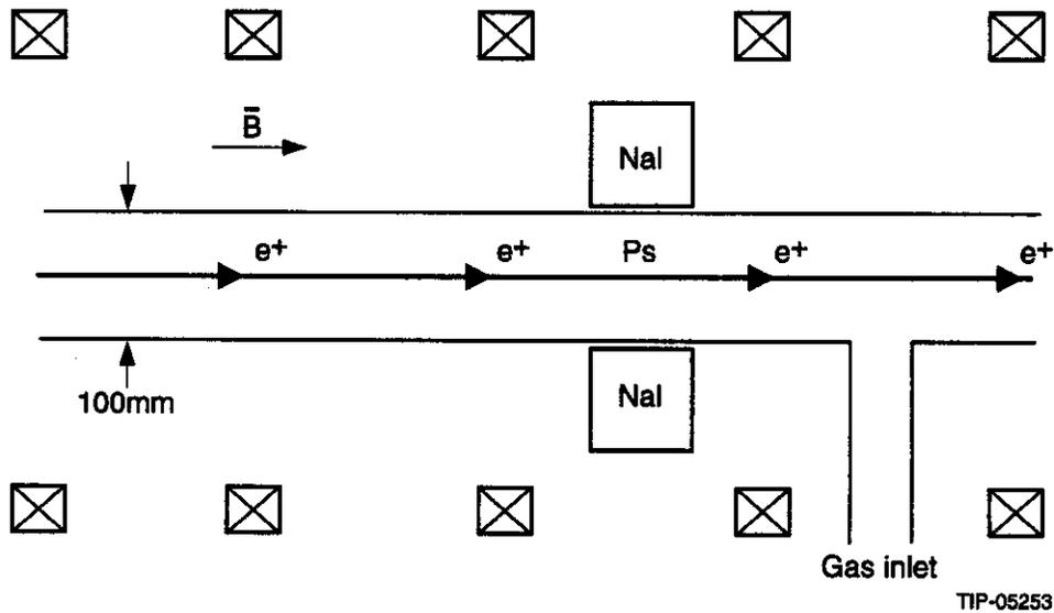
**Figure 2. The setup for the test experiment to determine the density of Hydrogen by monitoring the yield of Ps atoms.**
