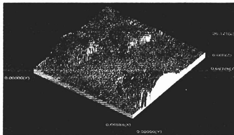
Fig. 11. Same as in Fig. 10, but with a greater magnification. Picture size:  $0.67 \times 0.66 \mu\text{m}^2$ . Three unbroken blisters are observed.
