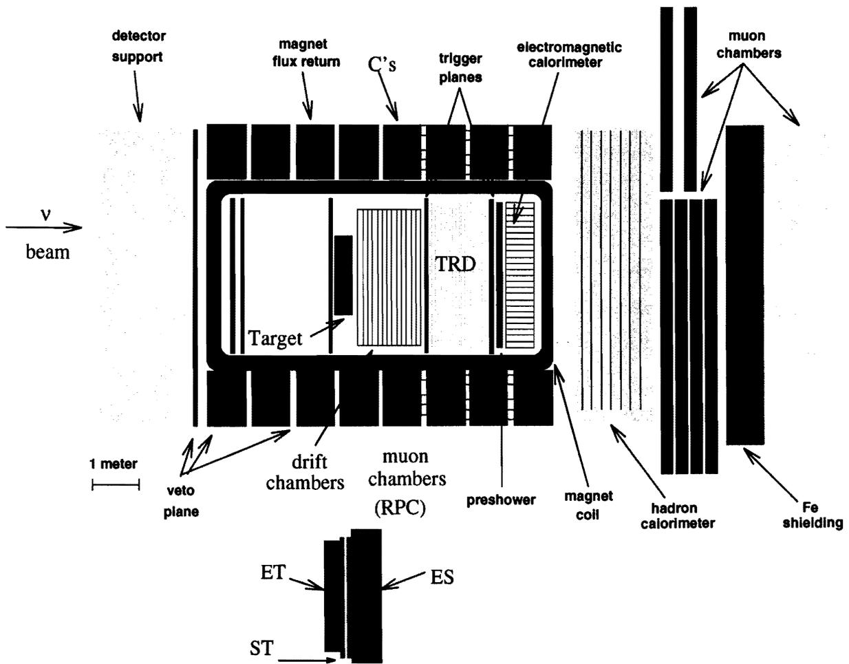
Figure 1: Schematic drawing of the TOP detector.
