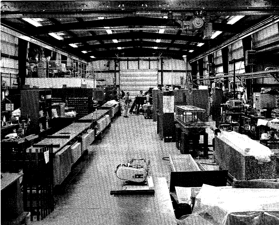
Fig. 7. Work in the Booster Laboratory. Girders with chokes and capacitors installed are at the left. Magnets are stacked at the far end, where Will Hanson and others are standing.
