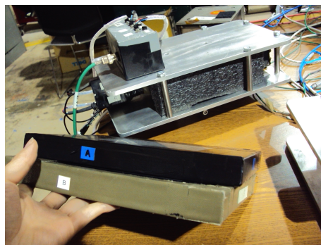
Figure 3: Photo of paddles used for the cosmic ray trigger, and the mechanical support for the paddle system.
