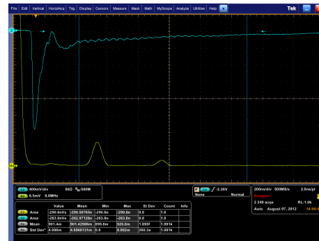
Figure 18: Driving the PCB splitter, we do not see any high frequency noise.
