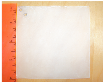
Figure 1. A typical plate used for our studies. The acrylic plate is clear, and the TPB coating has a milky appearance. Two holes were drilled into the plate for attachment to our testing apparatus (figure 2).
