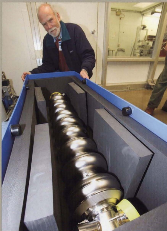
Barry Barish, Director of the ILC Global Design Effort, on tour of R&D areas at Fermilab inspecting a superconducting RF structure for potential use in the International Linear Collider.
