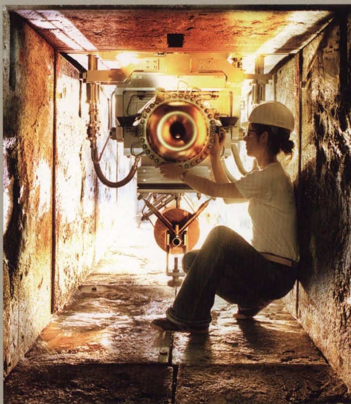
One of the two 'horns' of the NuMI beam line that focus the beam of particles for the MINOS neutrino experiment at Fermilab. The NuMI horn focuses short-lived particles called pions, which are generated when protons hit a target and decay to neutrinos (among other particles). The focusing is achieved using intense magnetic fields generated by 200,000-ampere pulses of electric current. (Photo credit Peter Ginter)
