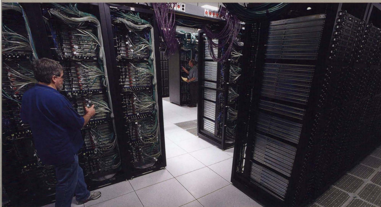
Dave Ritchie and Jack MacNerland at Wide Band's Grid Computing Center. In 1998 Fermilab began to employ clusters or "Farms" of low cost commodity PC's for Monte Carlo and experiment data reconstruction computing. Today the lab is using mostly commodity PC's, which provides lower cost computing through the purchase of approximately 1,000 units per year.
