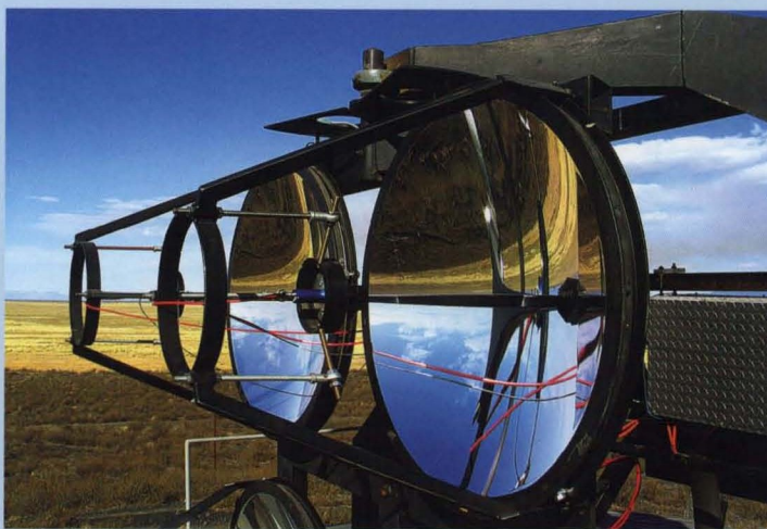
Mirrors of the Light Detection and Ranging (Lidar) system used for the atmospheric monitoring. Using Lidar systems, located near each fluorescence eye, the quality of air is monitored during the nights of fluorescence detector data taking. Also near the center of the array there are two central laser facilities, used to fire laser shots into the sky at night to calibrate the response of the nitrogen fluorescence detectors.
