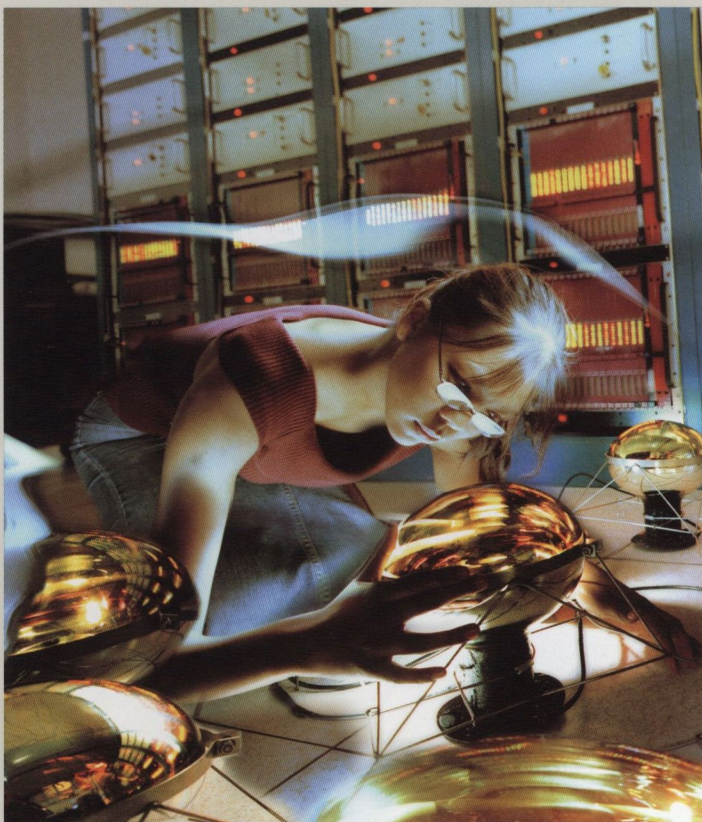
Jasmine Ma, a summer student working on the MiniBooNE experiment, inspects one of the phototubes that detects light from neutrino interactions. (Photo credit Peter Ginter)
