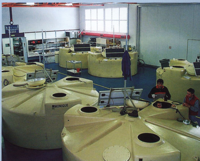
Preparing some of the 1,600 surface detector tanks in the Assembly Building prior to deployment for the Southern Auger array.
