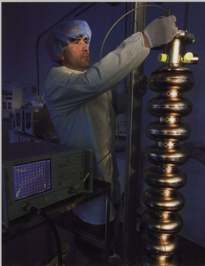
Scientist in a clean room at Fermilab testing a superconducting rf structure for potential use in the International Linear Collider.
