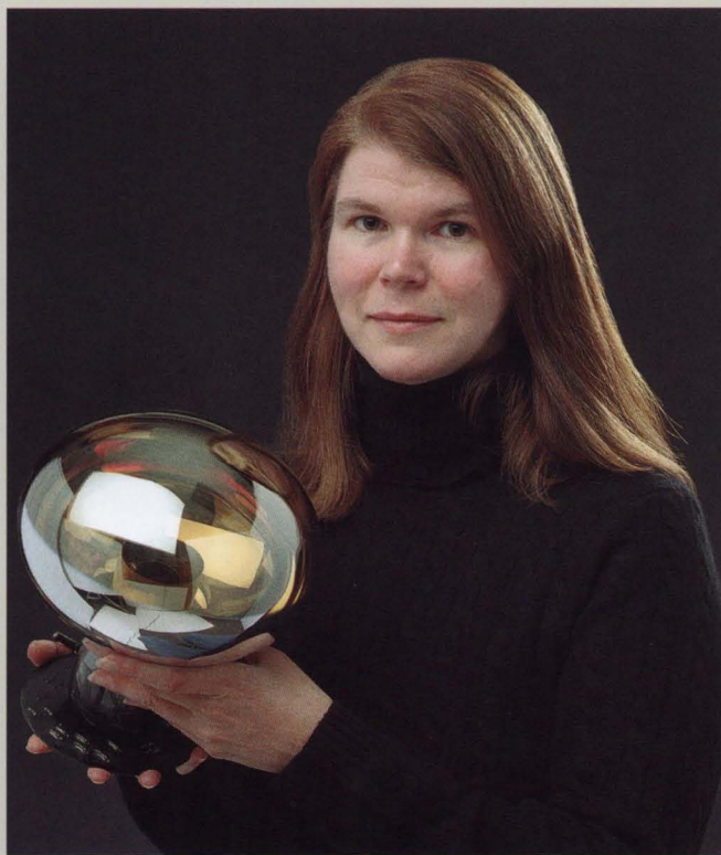
MiniBooNE cospokesperson Janet Conrad, Professor of Physics at Columbia University, holds one of the 1520 light sensors (called photomultiplier tubes) installed inside the MiniBooNE detector.
