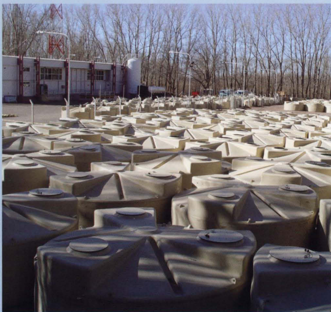
Some of the 1,600 surface detectors that are being prepared for deployment for the Southern Auger array to record showers of particles produced when cosmic rays strike the earth's atmosphere. The surface detectors are being spaced in the array about 1.5 kilometers apart.
