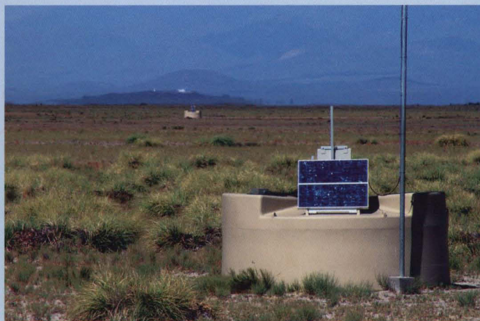
This photo shows two of the 1,600 surface detectors that are being deployed for the Southern Auger array. The surface detectors are spaced about 1.5 kilometers apart.
