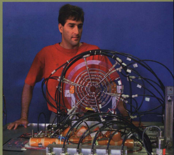
Steve Blusk of the University of Rochester views the cooling test stand for chip and ladder assemblies to be used at CDF.
