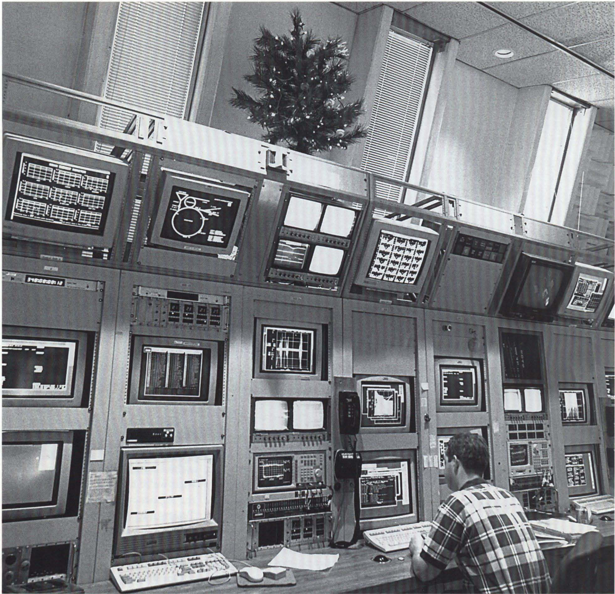
The Accelerator Division's Christmas tree, seen here in the Main Control Room, is actually a festive Tevatron monitor. The higher the luminosity, the faster the tree's lights blinked on and off. In 1995, the Tevatron collider routinely operated at 15 times its design luminosity.
