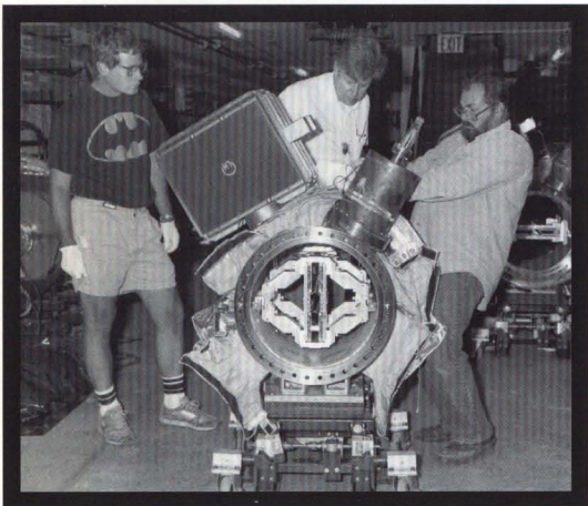
From the left, David McGinnis, Joel Misek and Henry Gusler prepare to install the stochastic cooling pick-up array in the Accumulator Ring of the Antiproton Source. The upgrade improved focusing of the antiproton core as the stack builds up.
