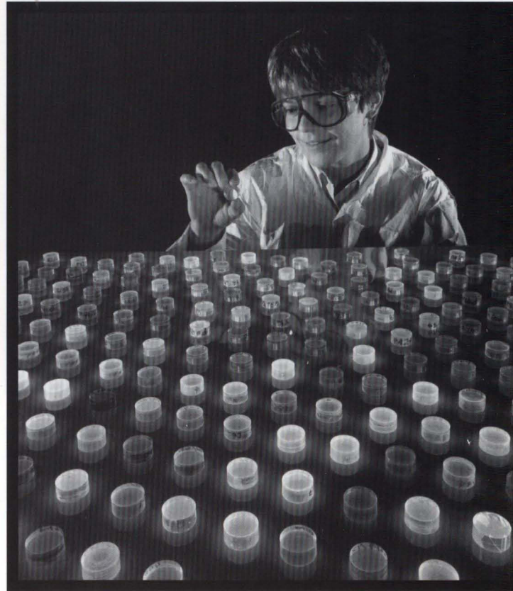
Anna Pla-Dalmau of the Research Division's Particle Detector Group examines a scintillator test sample. The small cylindrical samples, consisting of a polystyrene base doped with different fluorescent compounds, will be analyzed for various spectroscopic properties as scientists seek to find the most effective materials for the next generation of detectors.
