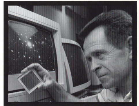
Merle Haldeman holds a two-inch square CCD chip for the Drift Scan Camera. Utilizing the largest CCD commercially available enables full sky coverage with reasonable resolution. The computer monitor displays an image of a field of galaxies typical of the data to be produced by the survey.
