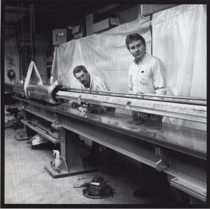
Scott Hawke (left) and Tom Anderson adjust the height of the detector carriage in the Source Projector Room at the Radiation Physics Calibration Facility. Different radioactive sources are placed behind the concrete wall and the carriage is moved remotely along the railroad tracks.
