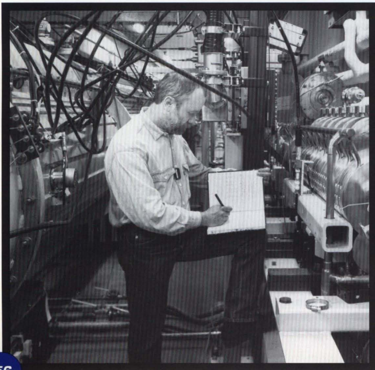
Mitchell Adamus checks the calibrations of the rf probes to determine the accelerating field inside the cavities of the new Linac. During the Tevatron shutdown in the summer of 1993, four tanks of the old Linac (to the left) will be removed and replaced by seven new accelerating modules operating at higher accelerating fields and higher frequency. The upgraded Linac will increase the output energy from 200 MeV to 400 MeV and reduce the transverse size of the beam in the Booster,
