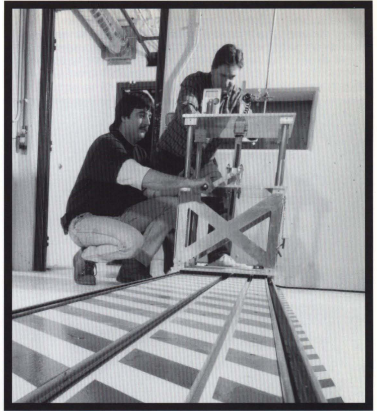
Scott Hawke (left) and Tom Anderson adjust the height of the detector carriage in the Source Projector Room at the Radiation Physics Calibration Facility. Different radioactive sources are placed behind the concrete wall and the carriage is moved remotely along the railroad tracks.
