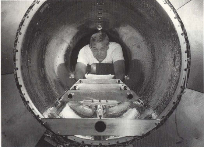
Inside the bore of the central tracking chamber of CDF, Michael Nurczyk performs alignment work on the ladder-like master fixture which is used to install supports for the vertex time projection chambers and the silicon vertex chambers.
