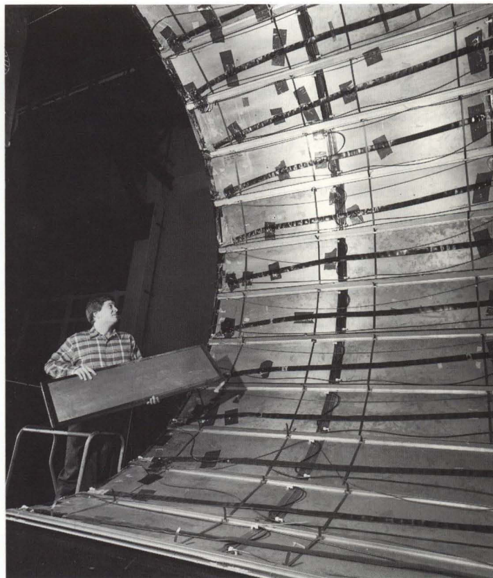
Dwarfed by the mammoth arch of completed chambers, Stephen Kublmann prepares to install another of the central preradiator chambers which sit behind the 1.0 radiation length CDF coil/cryostat.
