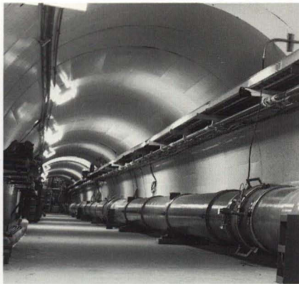
In this tunnel, a 275-foot long string of five 40-mm superconducting dipole magnets was successfully tested in August 1991.
