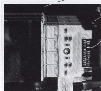
A close up of the readout end of the SVX detector's test wedge. The four ladders (layers) pictured contain microscopic strips that detect particle activity.
