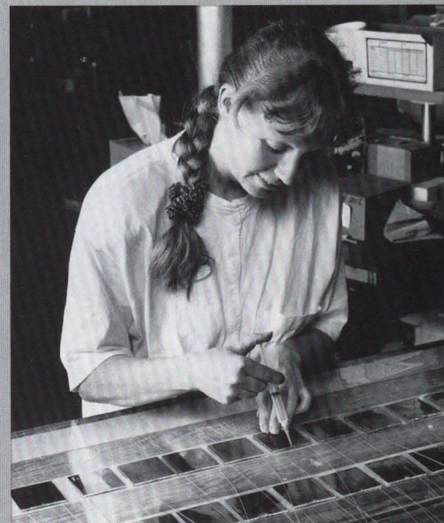
An amplifier sits apart from a silicon strip microvertex detector (SMD). The SMD detects charm and bottom particles as well as mesons and hadrons.
