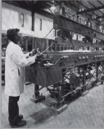
(Left) The Industrial Center Building contains presses for coil molding, collar keying, and for assembling and welding the helium containment vessels.
