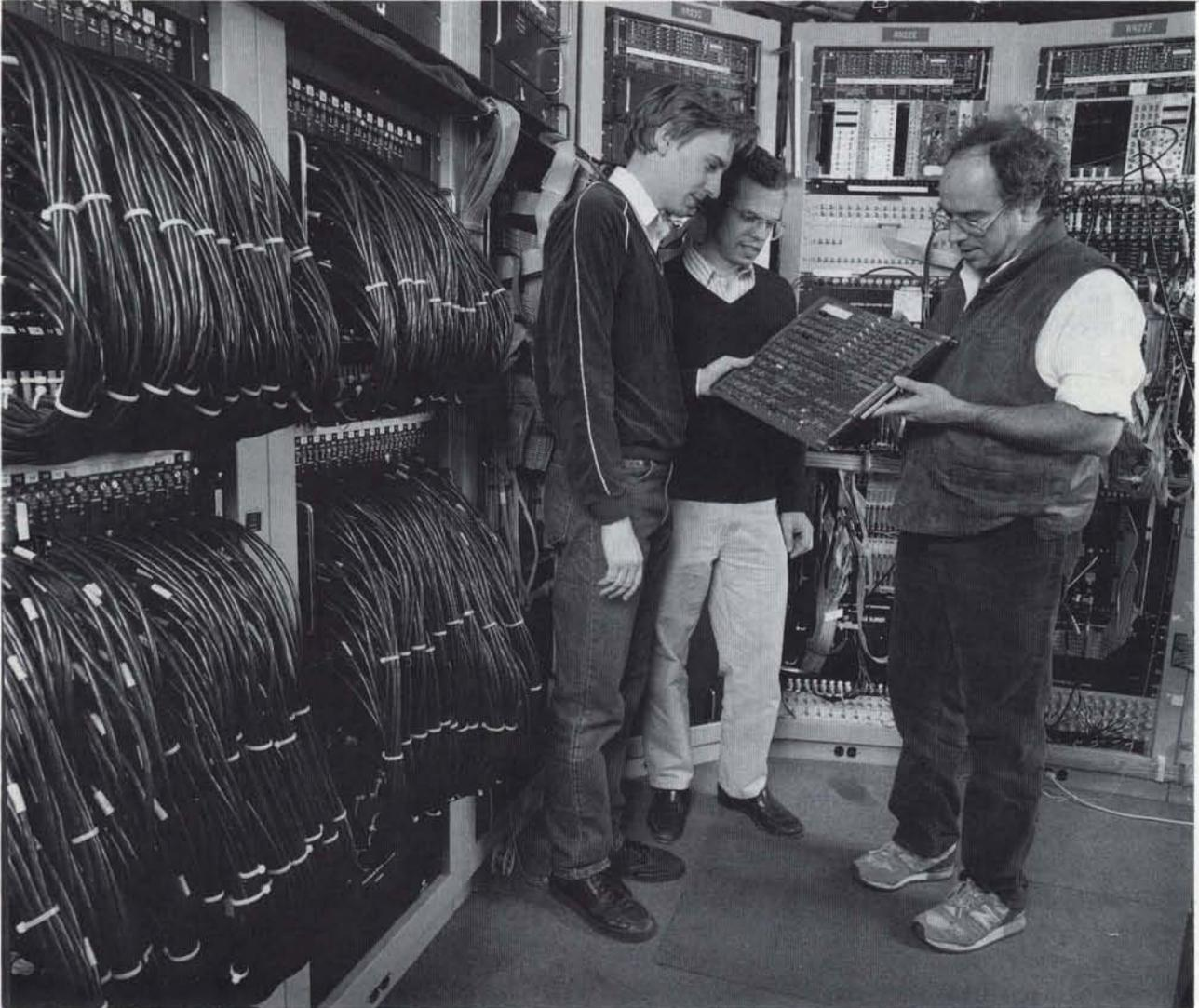
*Jay Hauser, Melvin Shochet, and Henry Frisch (from left to right) examine the special electronic sensing circuits and the many miles of cables in the trigger room of the CDF complex.*
