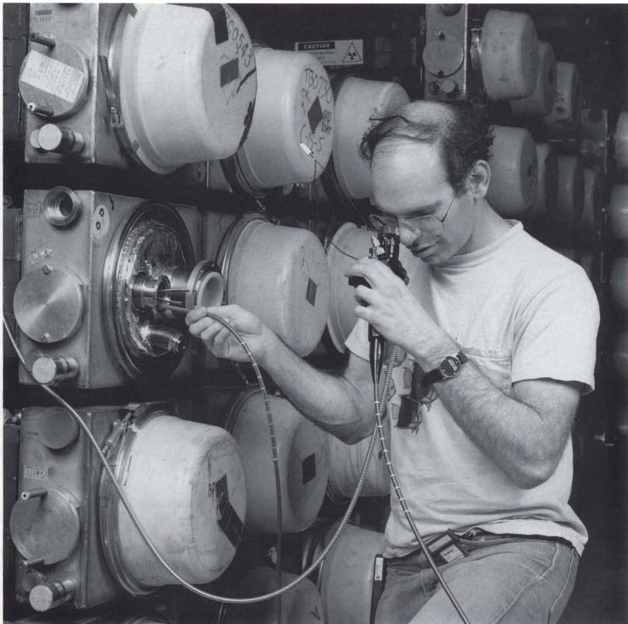
*Bruce Hanna examines the inside of a superconducting dipole magnet. Fermilab has pioneered the use of these "remote surgery" techniques for repairing sealed superconducting magnets.*
