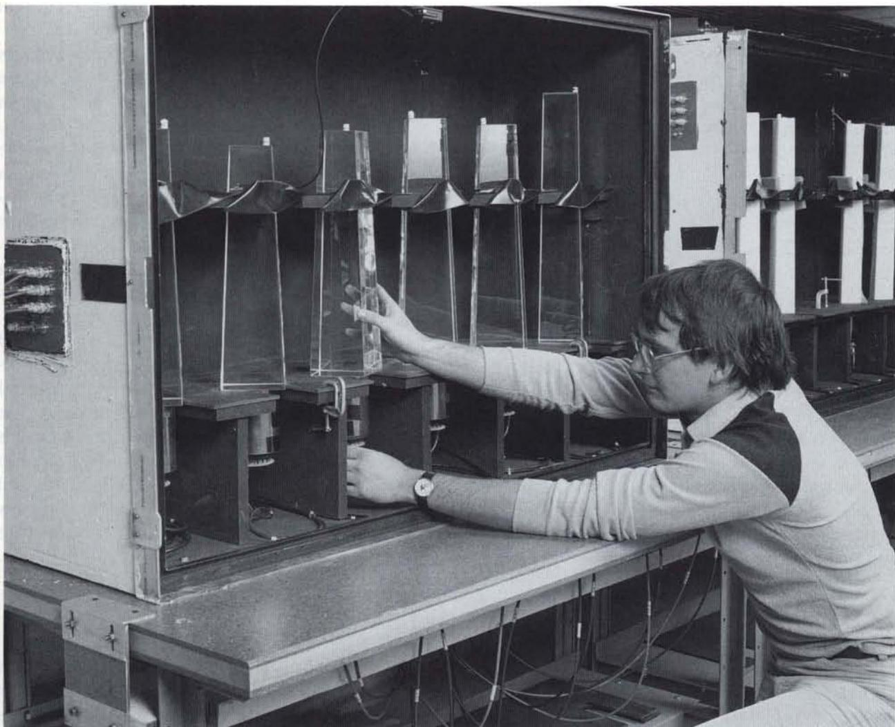
*Keith Gollwitzer works on the polished lead glass photon detectors used by E-760 in the Accumulator ring. Each block must be carefully calibrated before final installation.*
