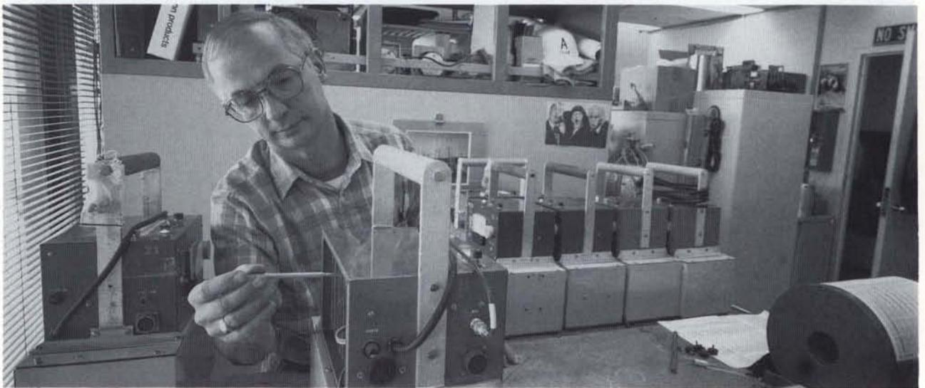
*Thomas Golaszewski of the Radiation Physics Technical Support Group performs the annual calibration of an area radiation monitor used by the Accelerator and Research Division. In 1989 this group, part of the Safety Section, continued its support role in providing reliable and well-calibrated safety instrumentation to the entire Fermilab community.*
