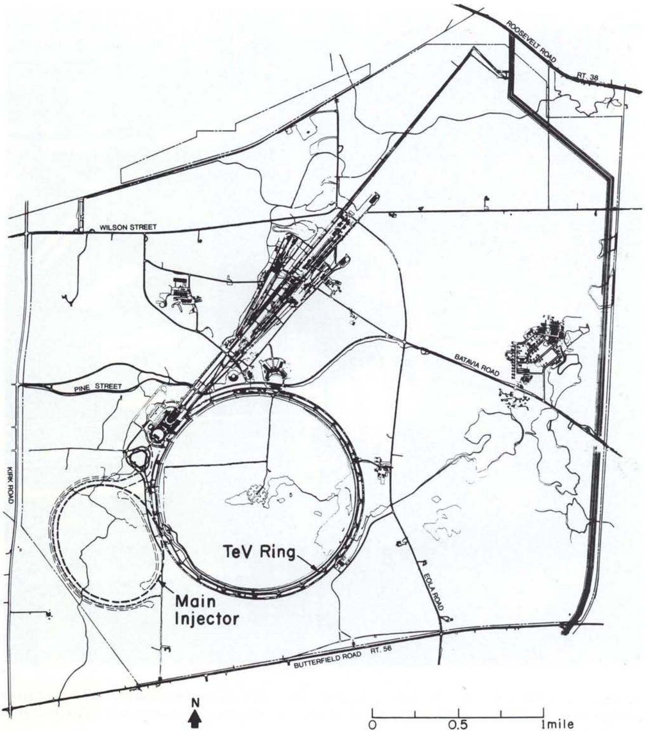
A schematic drawing shows the layout of the proposed Main Injector, the centerpiece of Fermilab III. The Main Injector is designed to be a 150 GeV accelerator which will replace the Main Ring, the original 200 GeV accelerator built at Fermilab nearly twenty years ago. Scientists working at Fermilab expect that Fermilab III will enable them to discover the top quark and perhaps observe the interaction of the elusive tau neutrino with ordinary matter.
