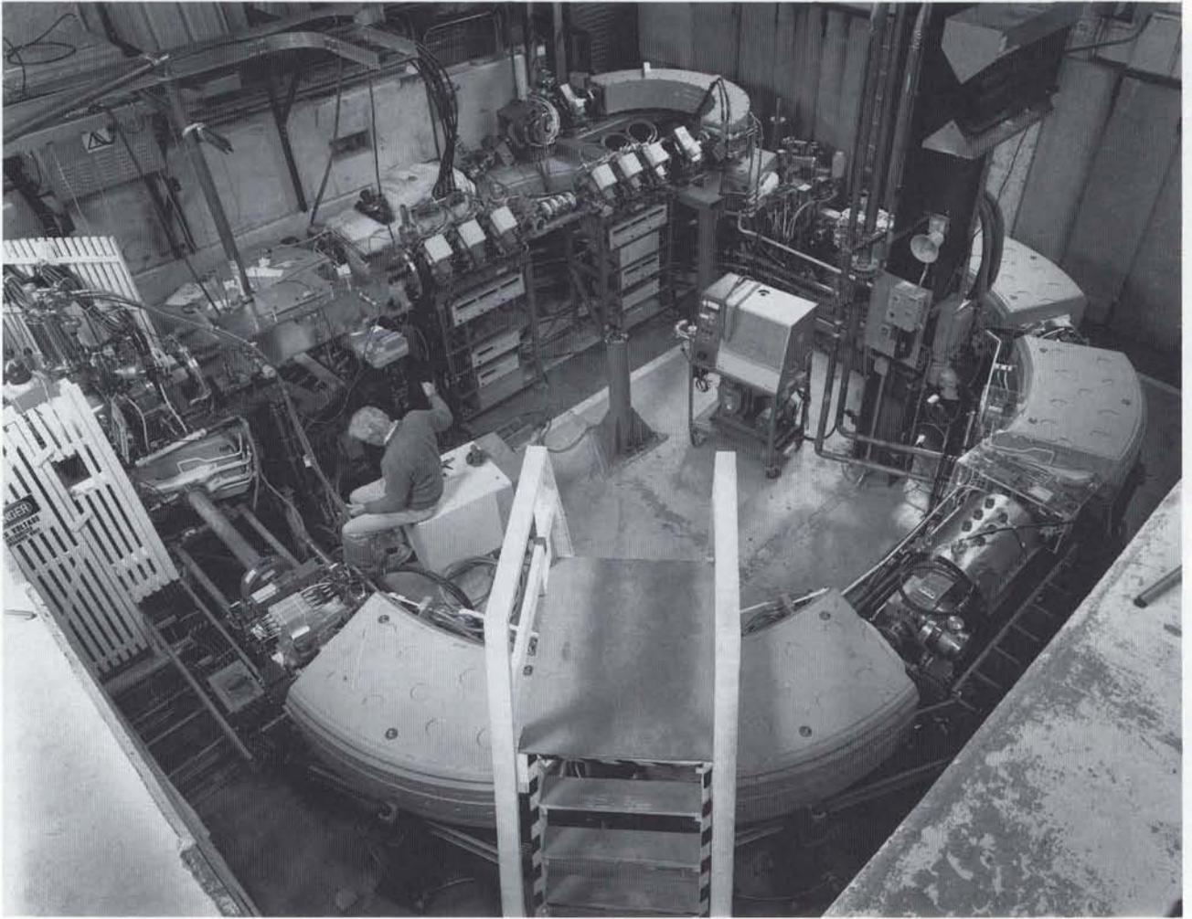
*This proton synchrotron, twenty feet in diameter, was designed and constructed by Fermilab for the Loma Linda University Medical Center where it will be used to treat cancer patients. This small accelerator provides a beam of protons whose energy, location, and intensity can be carefully controlled.*
