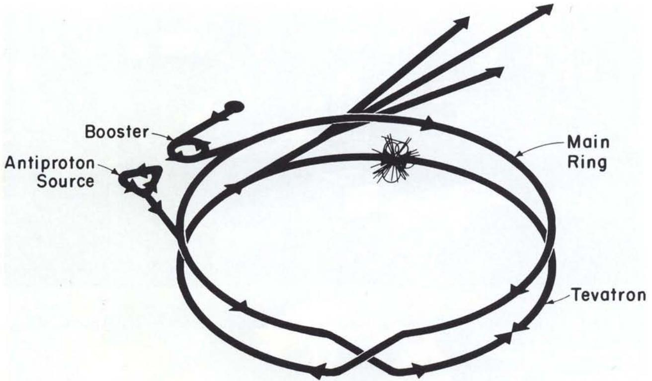
A schematic drawing shows the paths of the proton and antiproton beams in the Fermilab accelerator complex. The long journey, at close to the speed of light, must be controlled with extreme precision to effect collisions at the proper place within the detectors. Note that the protons and antiprotons circulate in opposite directions.
