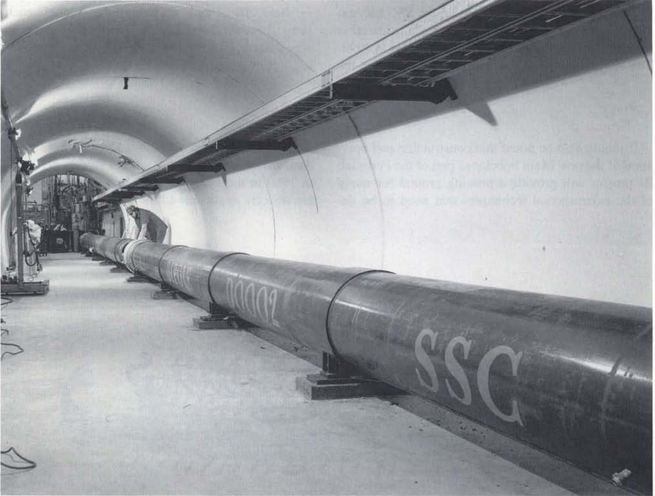
*As many as five SSC dipole magnets can be joined together in a string in this tunnel-like enclosure. They are then connected to and tested by utilizing the existing Tevatron cryogenic controls.*
