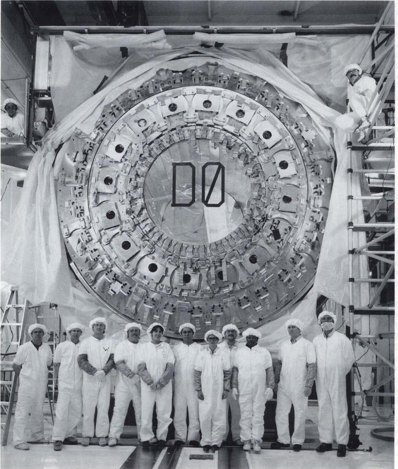
*Clean room workers pose with the central calorimeter modules for the D0 detector. Because of the extreme sensitivity of the device, it is essential that utmost cleanliness be maintained during its final assembly. The detector is approximately eighteen feet in diameter.*
