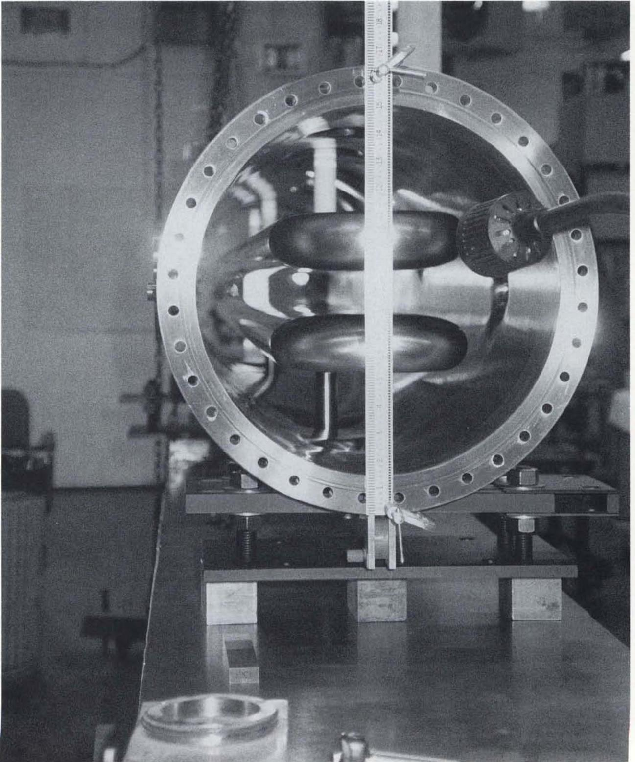
*A view of an electrostatic separator developed for the Fermilab III project.*
