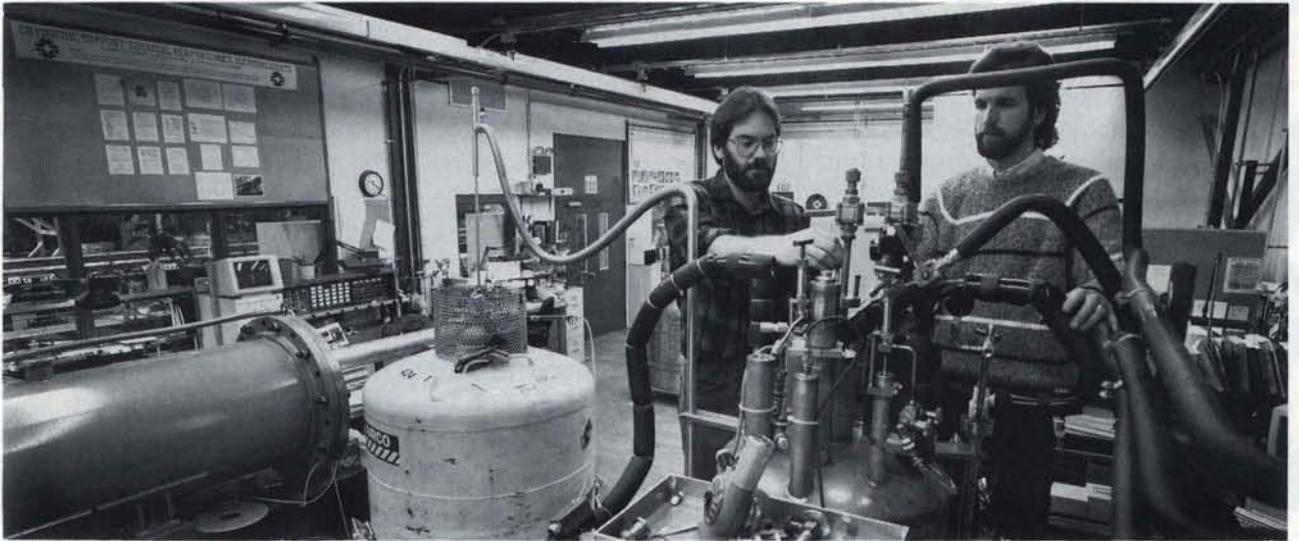
*Richard Kunzelman (left) and William Boroski of Technical Support conduct thermal performance measurements at the Engineering Laboratory Heat Leak Test Facility. The facility is commissioned to measure the performance of the superinsulation system for the SSC dipole magnets.*
