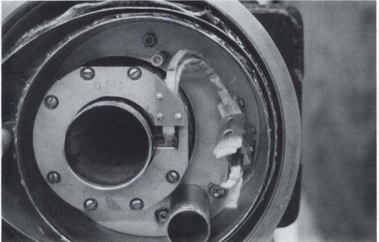
*An end view of a Tevatron magnet shows the superconducting current leads whose restraints were improved during the 1989 Tevatron repairs.*
