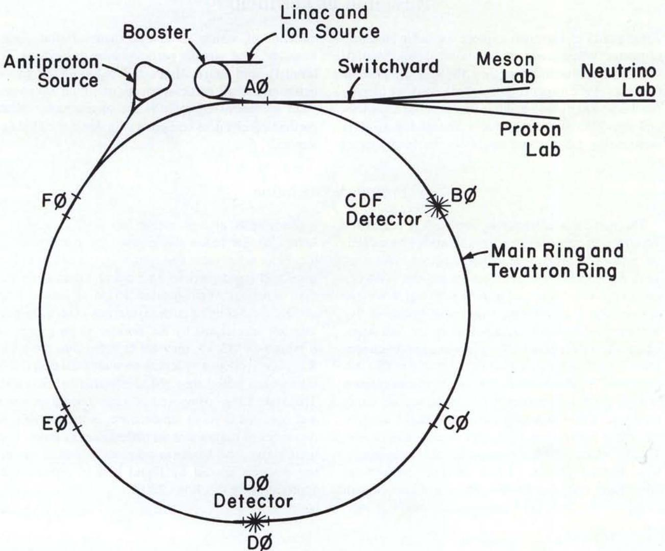
A schematic drawing shows the layout of various accelerators and experimental areas at Fermilab.
