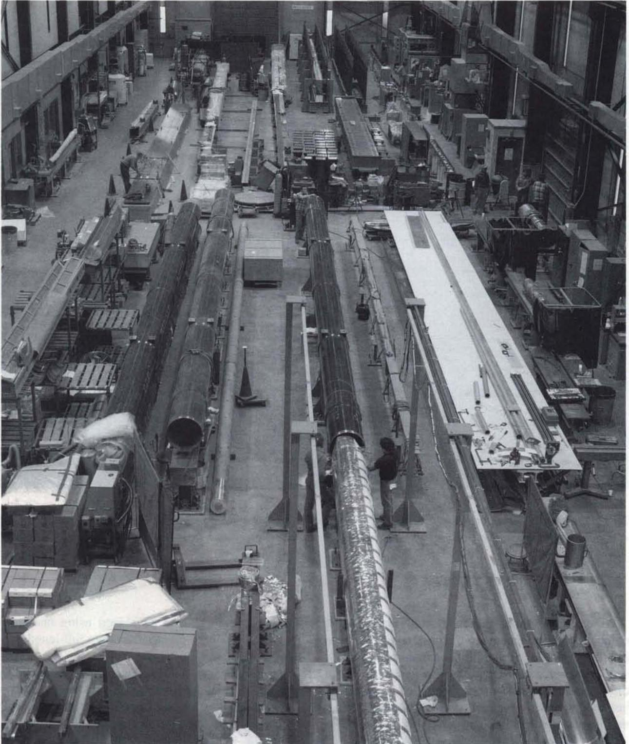
*The prototype SSC dipole magnets are being assembled in the Industrial Center Building.*
