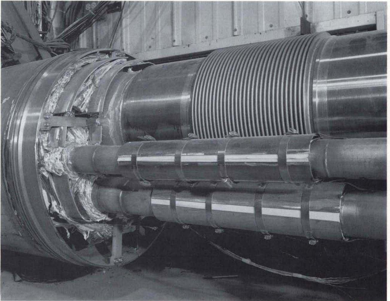
*This photograph shows the cryogenic connections at the end of a superconducting SSC dipole magnet. The cryogenic assembly and testing of the magnets take place at Fermilab.*
