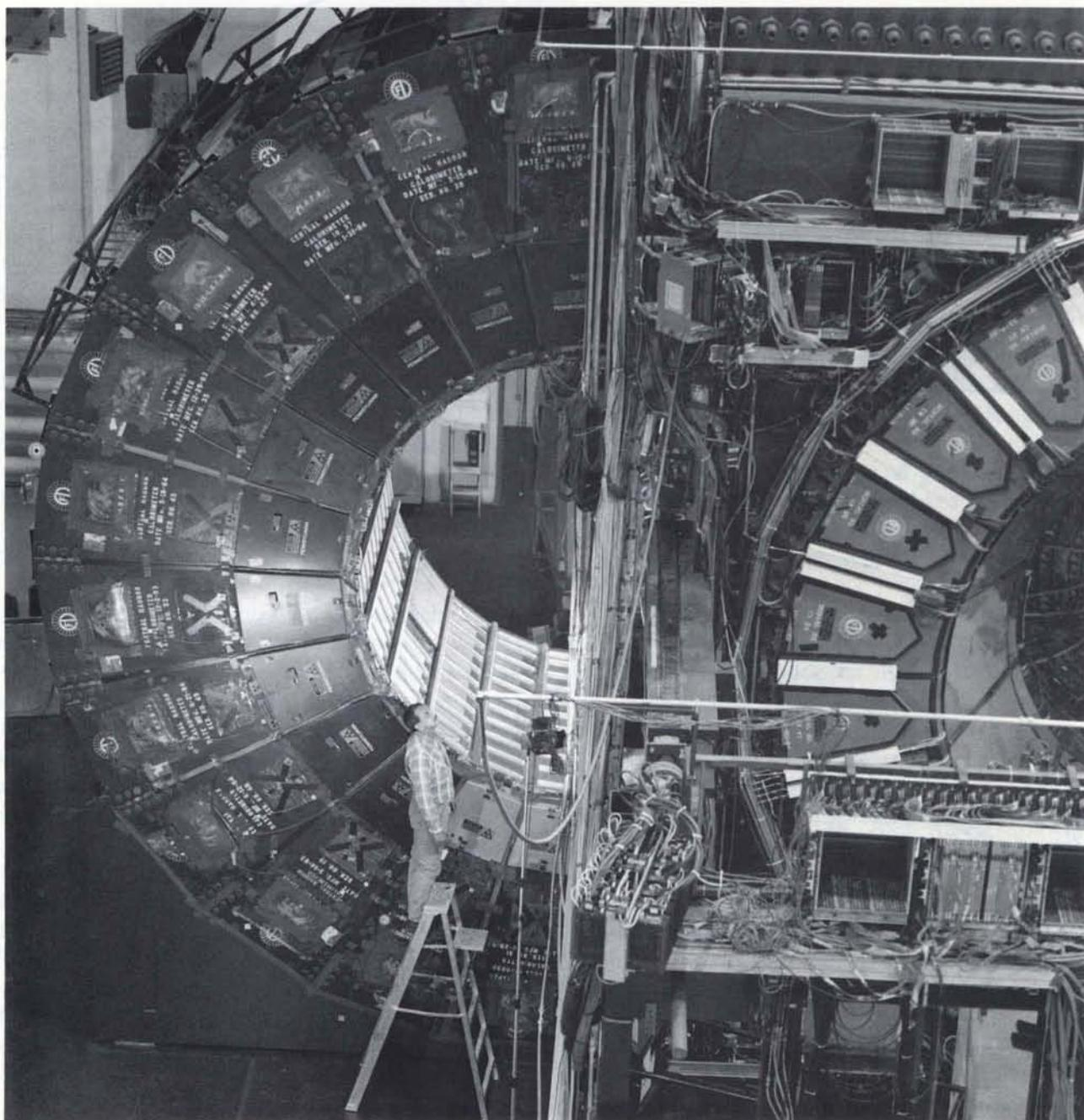
*A central calorimeter arch of the CDF detector is opened up for calibration and maintenance. These calorimeter modules wrap around the collision point and thus can measure the energy emitted in various directions from the proton-antiproton collisions.*
