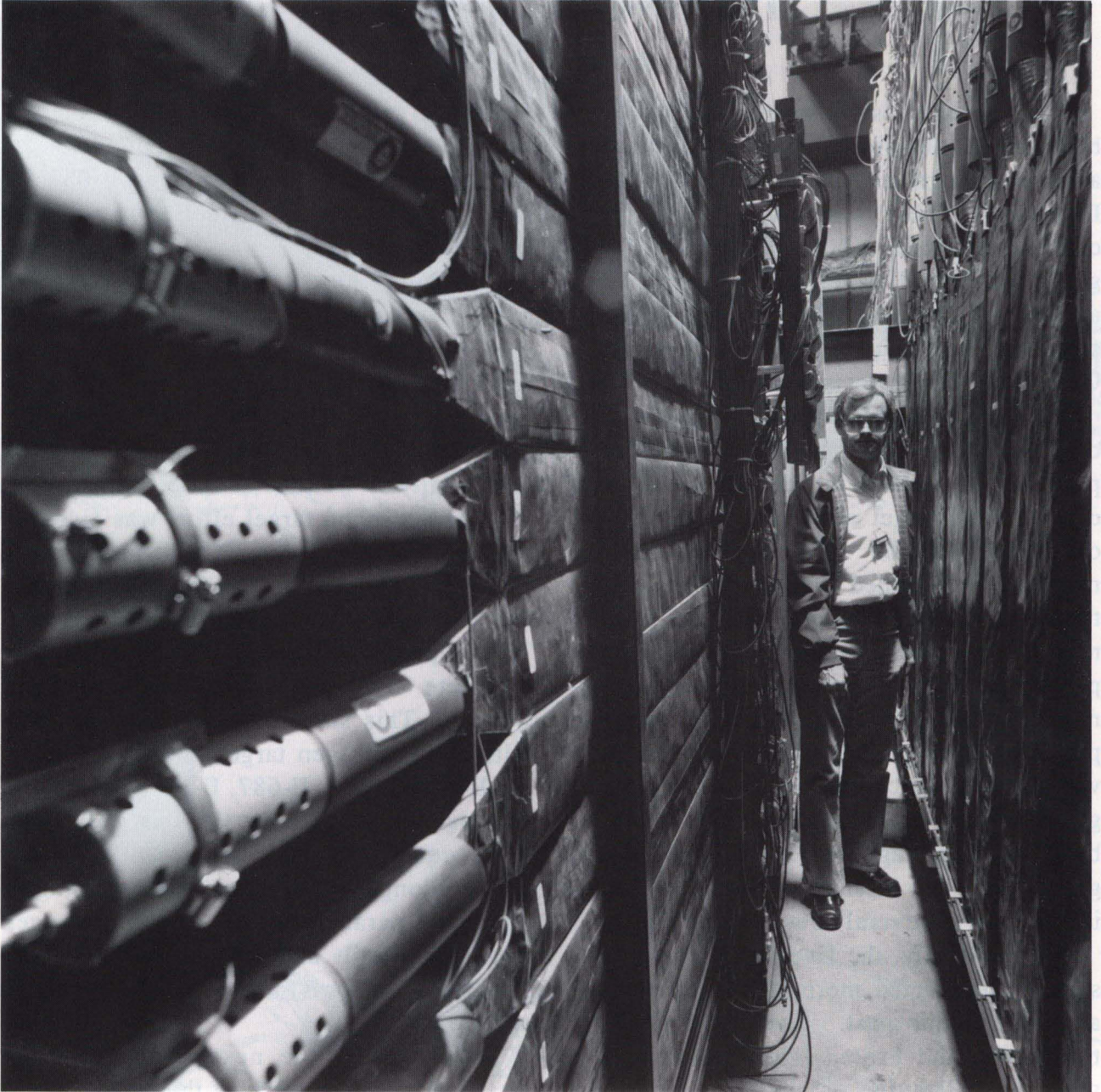
Banks of scintillation counters for E-705, placed in perspective by Merrill Jenkins (Fermilab).
