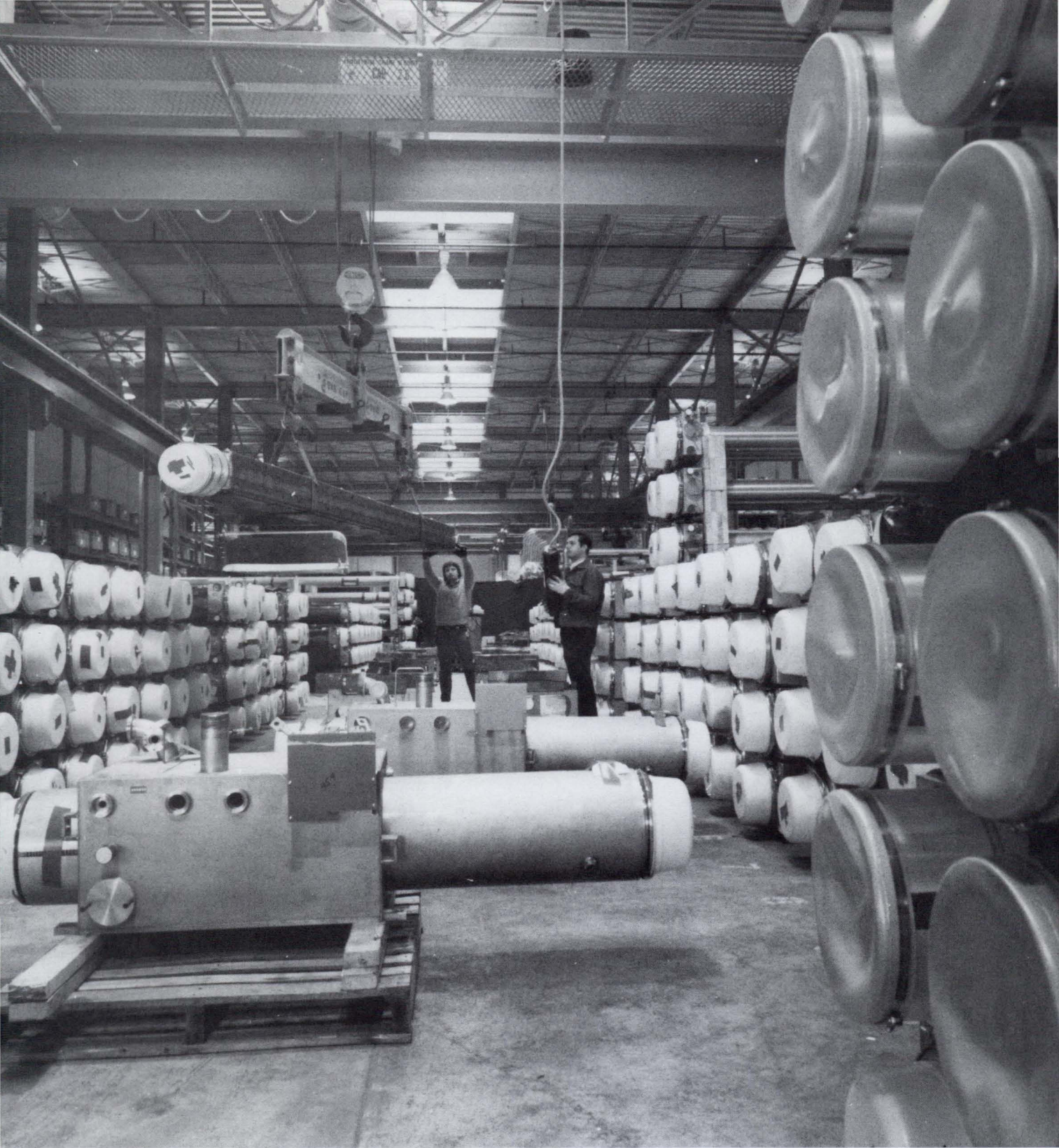
Gary Andrews and Norm Leja stacking Saver magnets and spool-pieces at Industrial 4 prior to installation in the Main-Ring tunnel.
