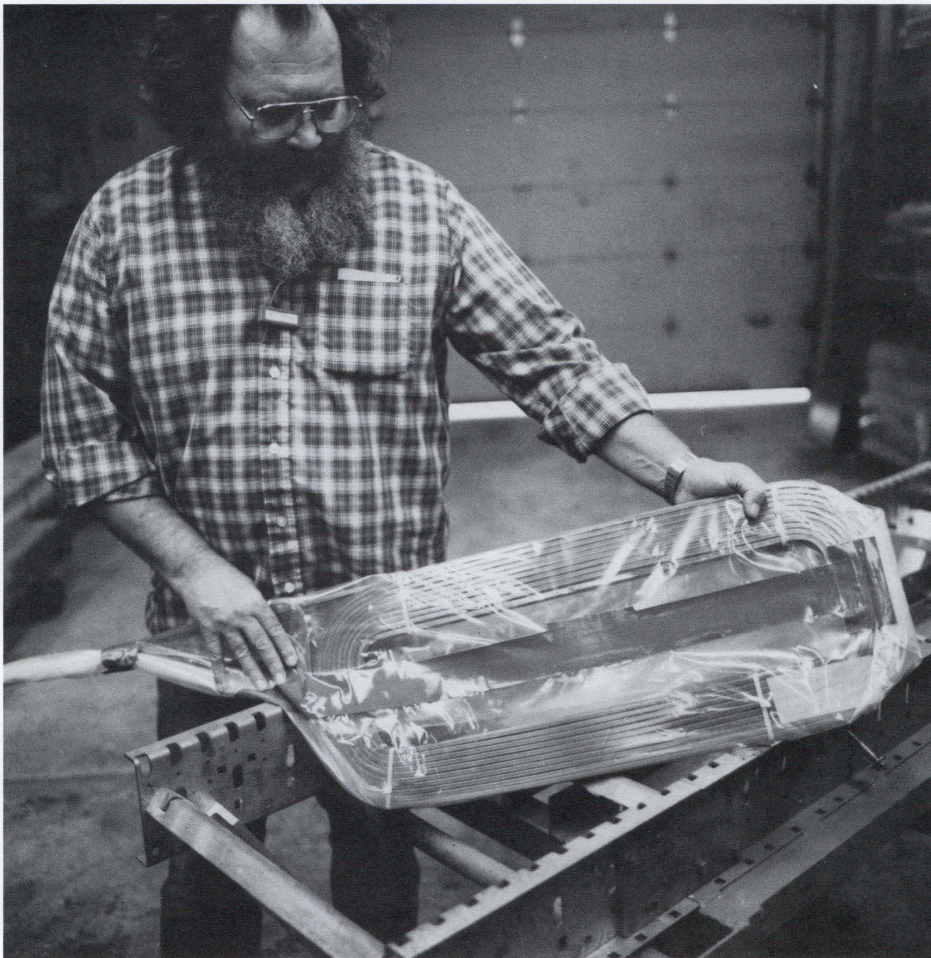
Jack Jagger with a coil for a TeV II 20-in. bump magnet.
