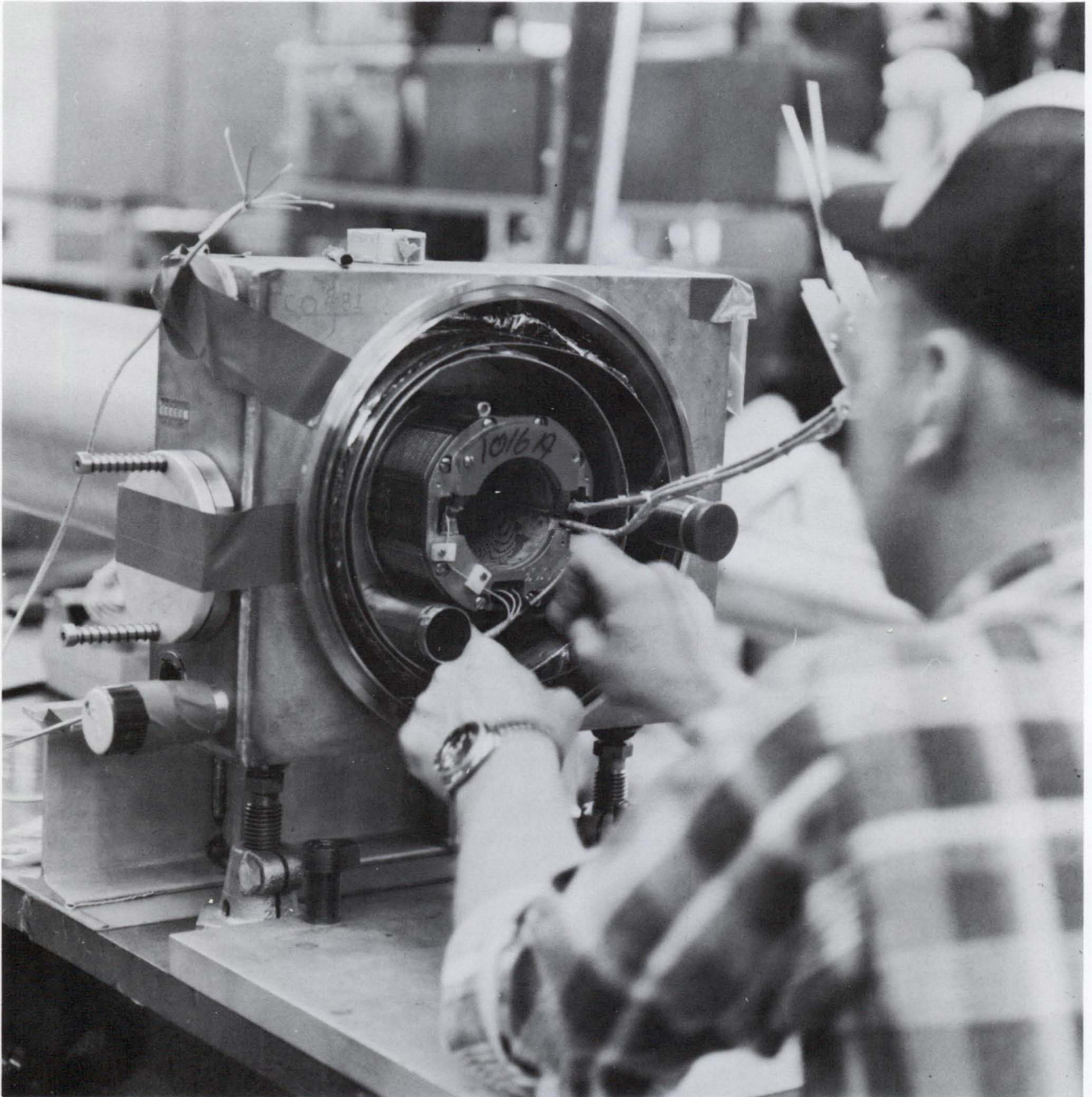
Final assembly of the end of a cryostat. The liquid nitrogen and two-phase helium tubes are just above Jerry Kucera's hands. The coil end can be seen inside the collared coil while the coil lead goes out over Jerry's shoulder.
