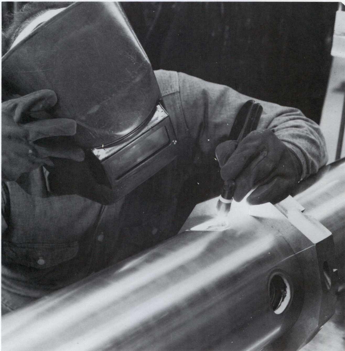
The coils will be mounted in a cryostat where they are kept cold. Here a welder is working on the mounting holes for anchor supports. These anchor supports hold the coil suspended inside the cryostat.
