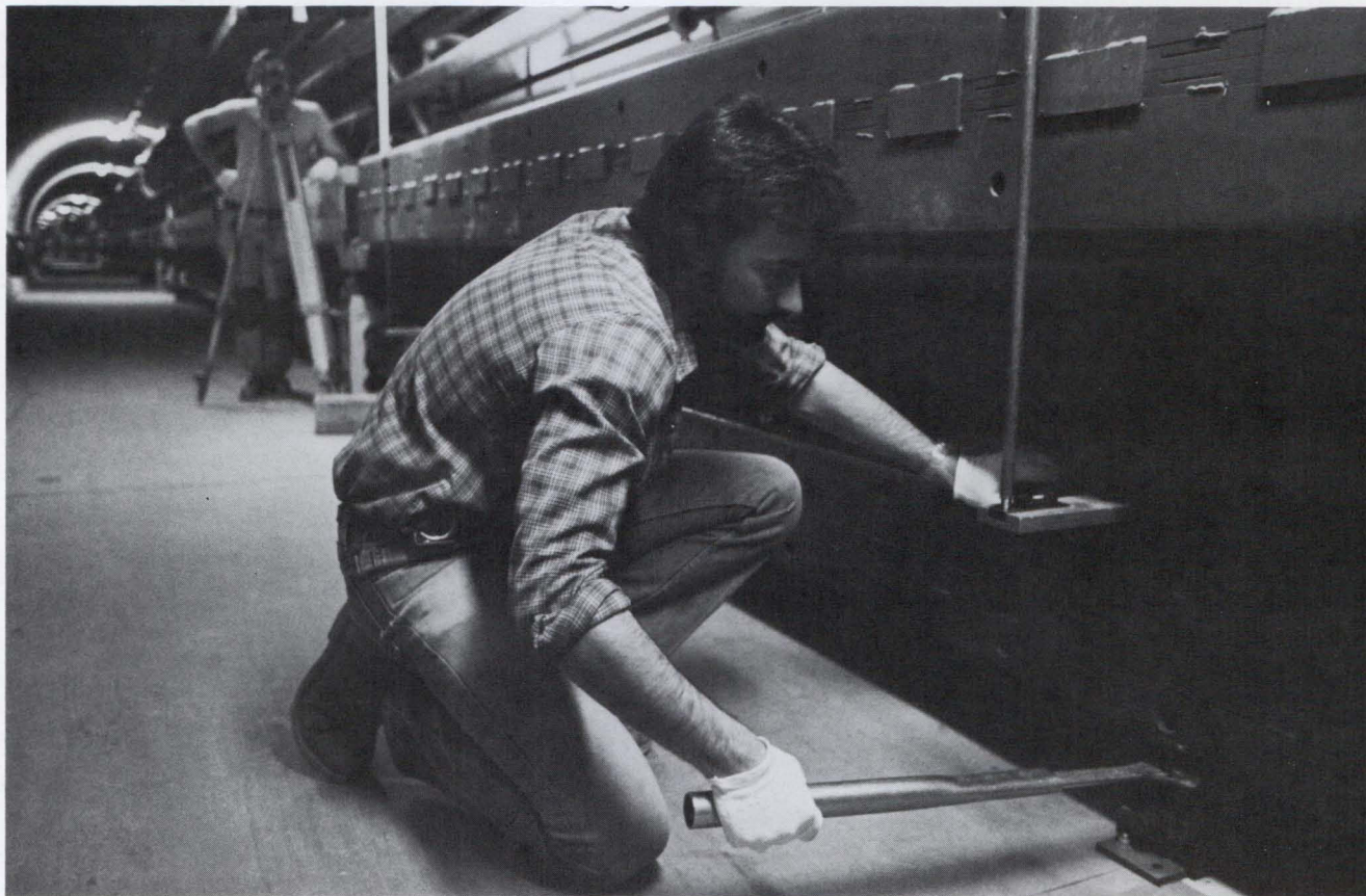
Gary Capola (kneeling) and Terry Guthke use surveying techniques to align a Saver magnet to within a few thousandths of an inch.
