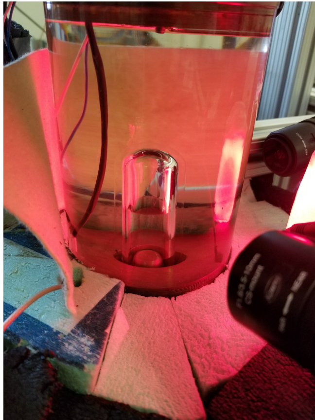
Figure 4. A photograph of the active part of the bubble chamber inside the temperature-control bath. The camera's view is at right angles to capture perpendicular views of bubbles for simple position reconstruction. This image was taken while filling the chamber with C_3F_8 ; the surface of the liquid is visible about halfway up the visible part of the bubble chamber.
