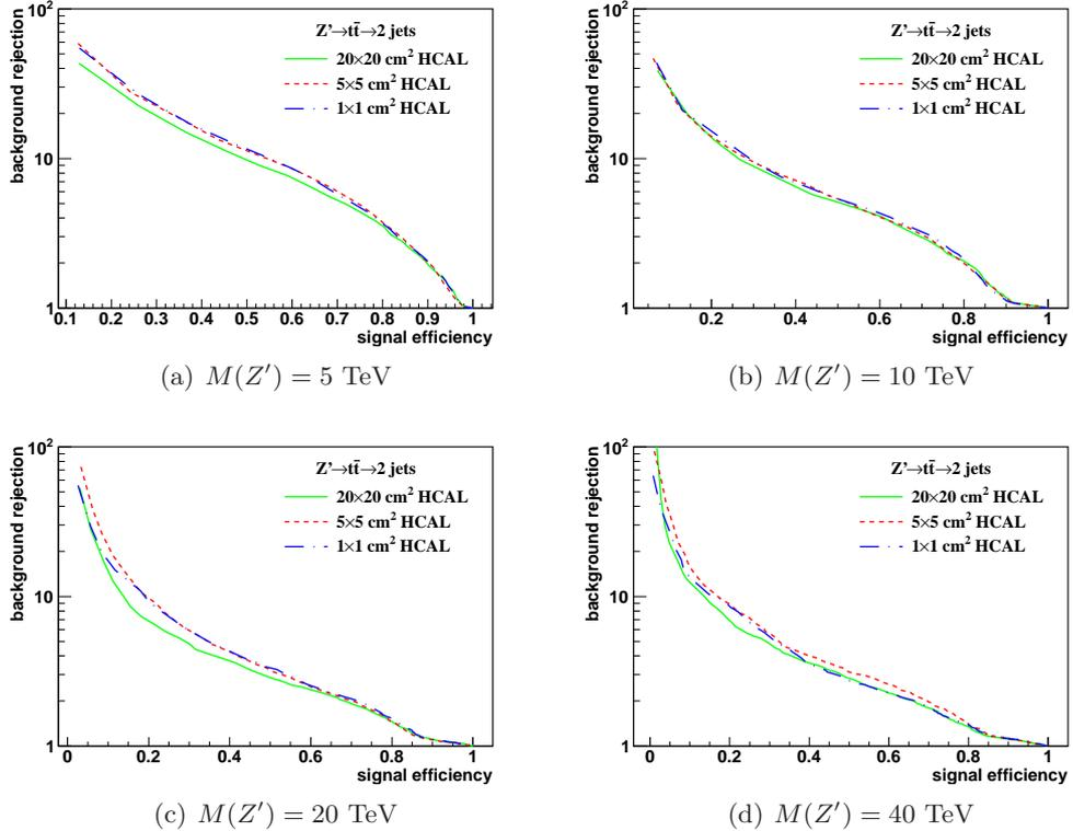
Figure 10: The ROC curves of soft drop mass selection for  $\beta = 2$  with resonance masses of 5, 10, 20 and 40 TeV. Three different detector cell sizes are compared:  $20 \times 20$ ,  $5 \times 5$  and  $1 \times 1 \text{ cm}^2$ . The signal (background) process is  $Z' \rightarrow t\bar{t}$  ( $Z' \rightarrow q\bar{q}$ ).
