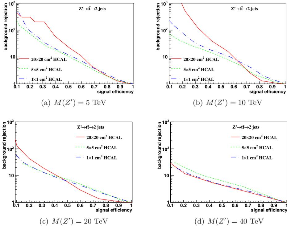
Figure 14: Signal efficiency versus background rejection rate using  $\tau_{32}$ . Resonance masses of (a) 5 TeV, (b) 10 TeV, (c) 20 TeV and (d) 40 TeV are shown here. In each figure, the three ROC curves correspond to different HCAL cell sizes.
