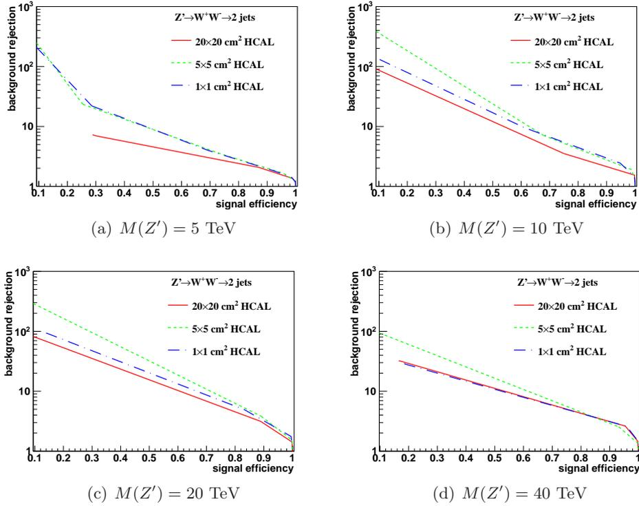
Figure 16: Signal efficiency versus background rejection rate using  $C_2^1$ . The resonance masses of (a) 5 TeV, (b) 10 TeV, (c) 20 TeV, and (d) 40 TeV are shown here. In each figure, the three ROC curves correspond to different detector sizes.
