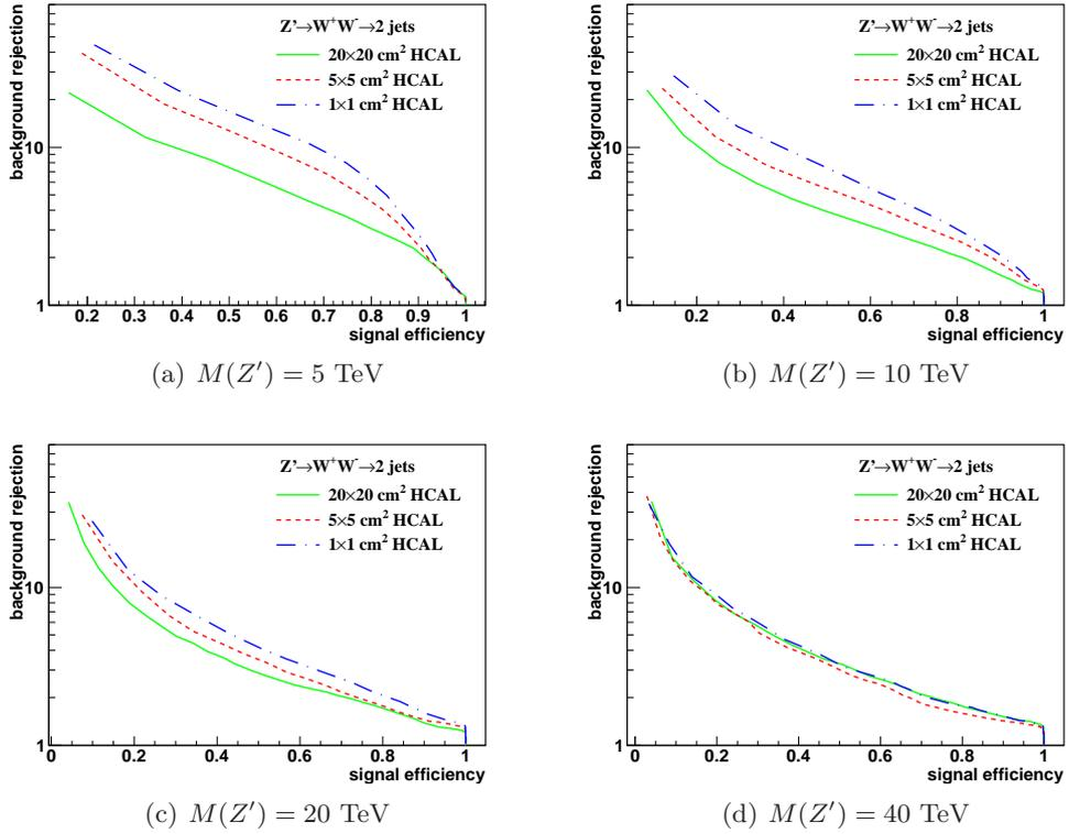
Figure 4: The ROC curves of soft drop mass selection for  $\beta=0$  with resonance masses of 5, 10, 20 and 40 TeV. Three different detector cell sizes are compared:  $20 \times 20$ ,  $5 \times 5$ , and  $1 \times 1 \text{ cm}^2$ . The signal (background) process is  $Z' \rightarrow WW$  ( $Z' \rightarrow q\bar{q}$ ).
