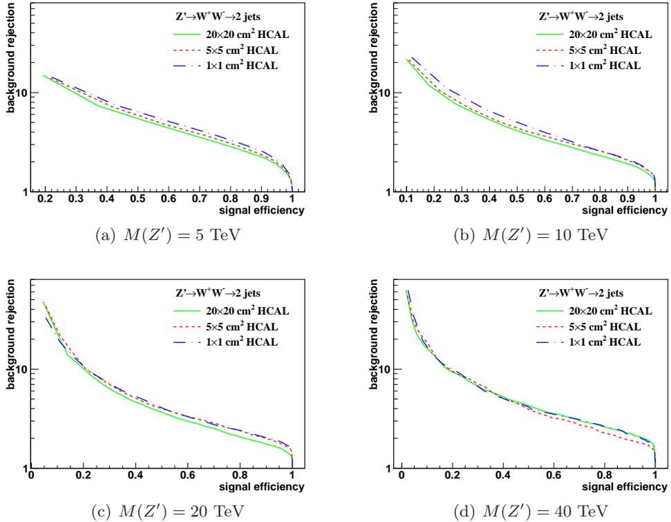
Figure 8: The ROC curves of soft drop mass selection for  $\beta = 2$  with resonance masses of 5, 10, 20 and 40 TeV. Three different detector cell sizes are compared:  $20 \times 20$ ,  $5 \times 5$ , and  $1 \times 1 \text{ cm}^2$ . The signal (background) process is  $Z' \rightarrow WW$  ( $Z' \rightarrow q\bar{q}$ ).
