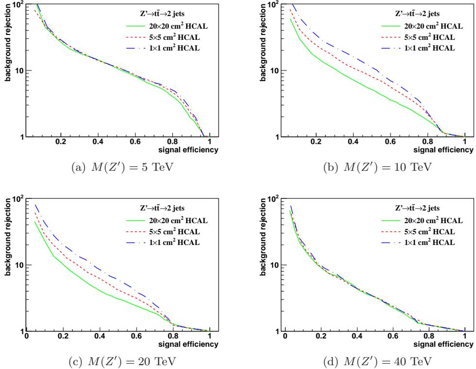
Figure 6: The ROC curves of soft drop mass selection for  $\beta=0$  with resonance masses of 5, 10, 20 and 40 TeV. Three different detector cell sizes are compared:  $20 \times 20$ ,  $5 \times 5$ , and  $1 \times 1 \text{ cm}^2$ . The signal (background) process is  $Z' \rightarrow t\bar{t}$  ( $Z' \rightarrow q\bar{q}$ ).
