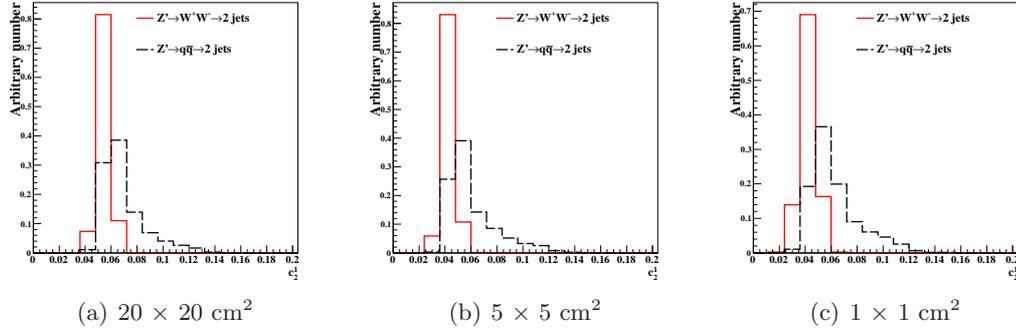
Figure 15: Distributions of  $C_2^1$  with  $M(Z') = 20 \text{ TeV}$  for different detector granularities. Cell sizes of  $20 \times 20$ ,  $5 \times 5$ , and  $1 \times 1 \text{ cm}^2$  are shown here.
