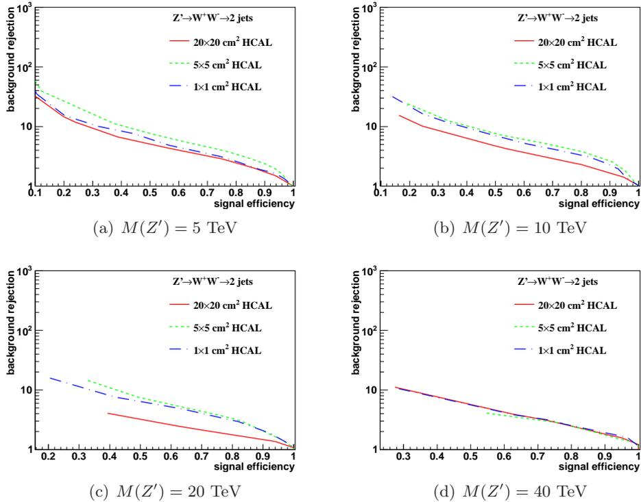
Figure 12: Signal efficiency versus background rejection rate using  $\tau_{21}$ . Resonance masses of (a) 5 TeV, (b) 10 TeV, (c) 20 TeV and (d) 40 TeV are shown here. In each figure, the three ROC curves correspond to different cell sizes.
