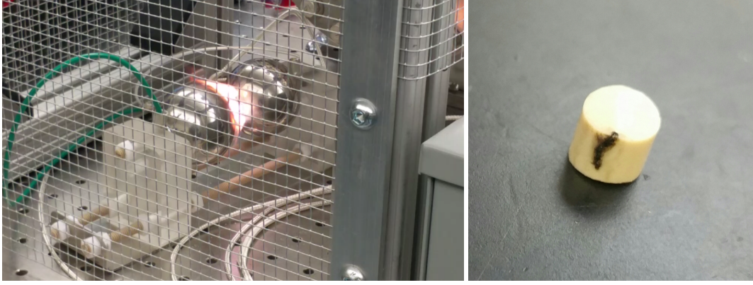
Figure 3. Left: anti-static UHMW tested in air and failing through sparking and excessive heating at \leq 10 kV; Right: picture of PEEK post that had a destructive spark leave a track along the side.
