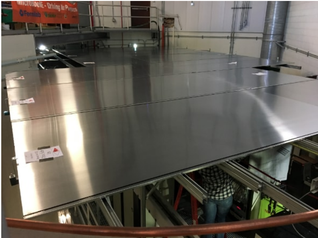
Figure 18: Completed MicroBooNE CRT top plane.
