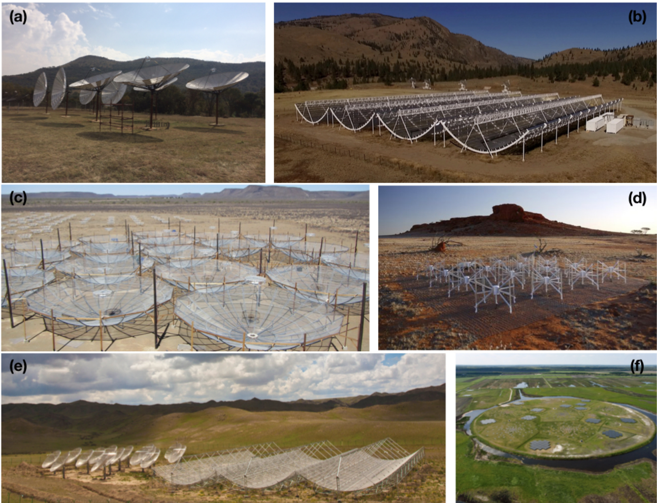
FIG. 18. A sample of relevant 21 cm interferometric experiments currently fielded: (a) 8-element HIRAX prototype array operating at 400–800 MHz [160]; (b) CHIME experiment operating at 400–800 MHz [181]; (c) HERA [182] operating at 50–250 MHz with PAPER [183] in the background; (d) MWA operating at 80–300 MHz [184]; (e) Tianlai [185] operating at 700–800 MHz; (f) LOFAR [186] operating at 10–230 MHz. EDGES [187] is not included because it is targeting a global signal. LEDA is relevant but not pictured [188].
