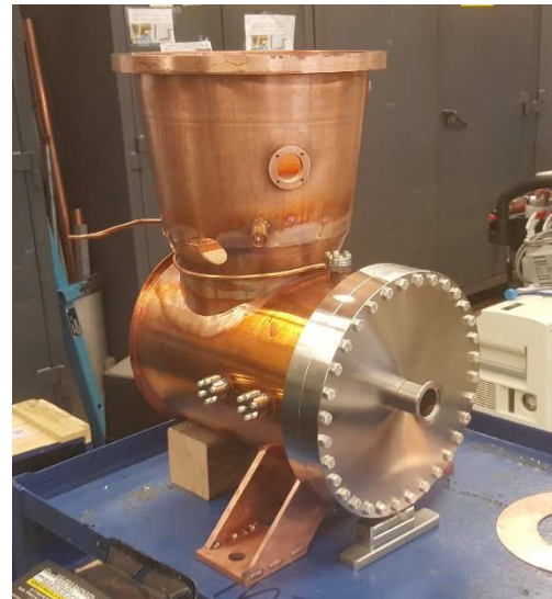
Figure 13 : The partially assembled cavity.
