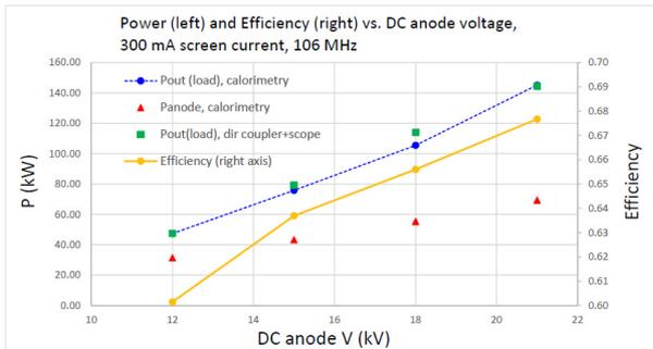
Figure 5: Output power, power dissipated in the anode, and efficiency for Y567b tests at 106 MHz.
