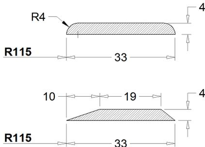
Figure 4: Initial and final shim designs. All dimensions in mm.
