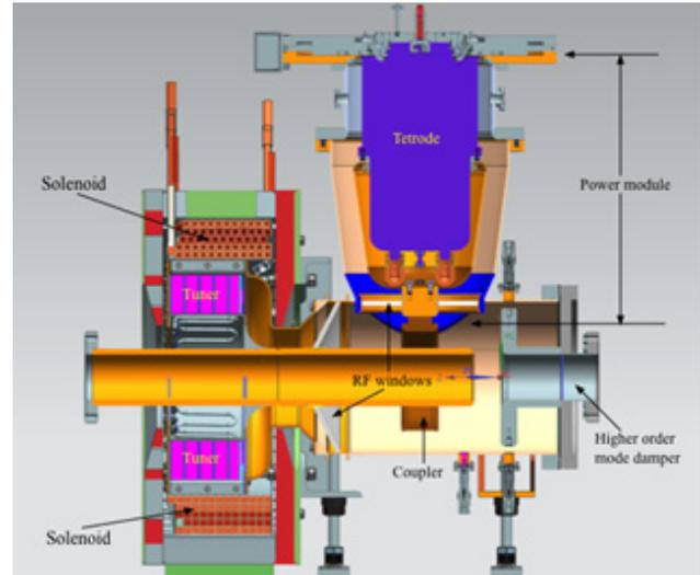
Figure 1: Model of the finalized cavity design. The length is 33.21 in. from flange to flange.
