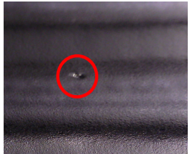
Fig. 10. Example defect on side wall of Vendor A cavity after 275 micron EP.
