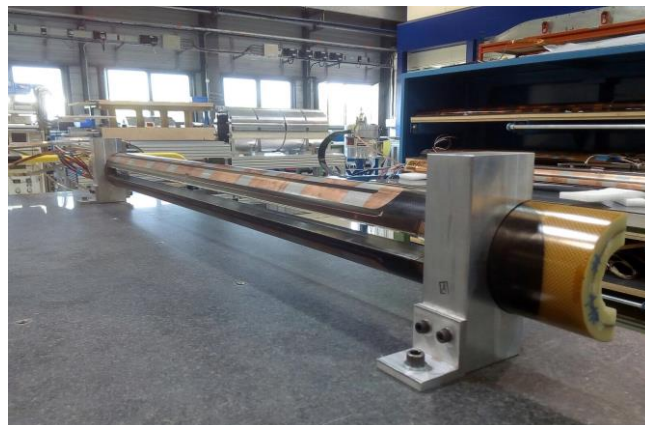
Fig. 1. HL-LHC 11 T Dipole coil fixed on the marble reference surface, ready for geometrical measurements.
