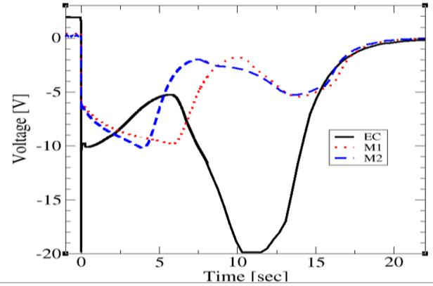
Fig. 6. SSU Training quench at 280 A taken at RAL.
