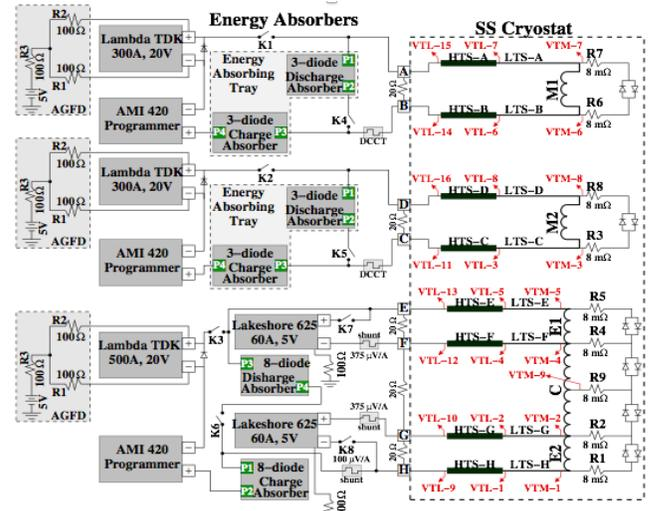
Fig. 3. Spectrometer Solenoid Powering Circuit.
