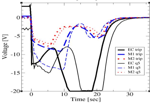
Fig. 8. SSD coil voltage signal evolution for quench number 5 and the trip event that occurred after q5. Current value for M1 for q5 event was 198 A and for the trip event was 195 A.
