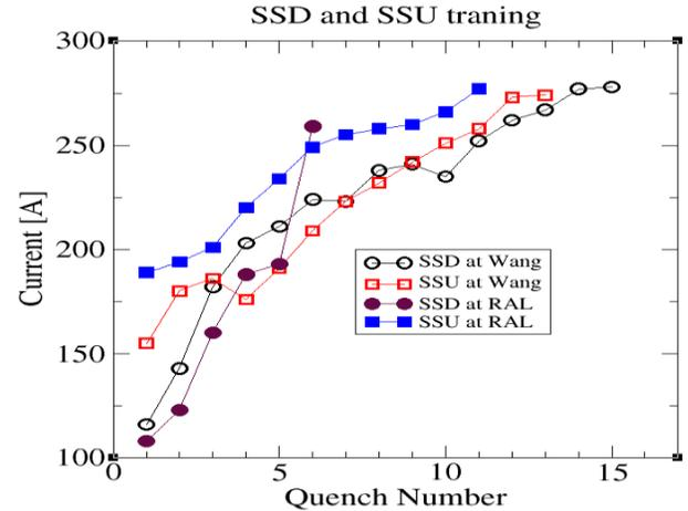
Fig. 4. Quench Training of SSU and SSD. After the last quench of SSD the M1 circuit was opened.
