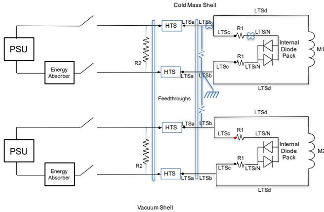
Fig. 5. M1 and M2 circuits after quench number 6.
