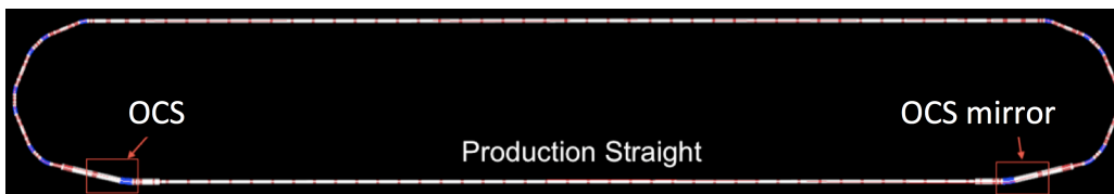
Figure 7. The decay ring layout. Pions are injected into the ring at the Orbit Combination Section (OCS). Similarly, extraction of pions and muons at the end of the production straight is done using a mirror image of the OCS.
