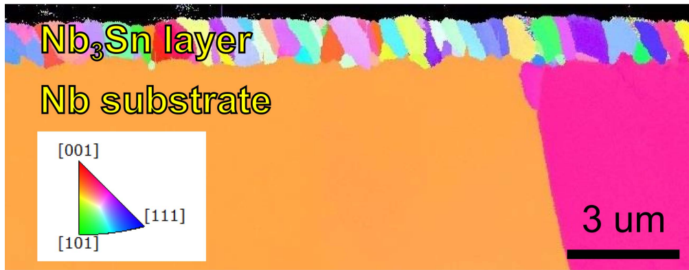
Figure 24. EBSD image of a cross section of a \text{Nb}_3\text{Sn} coating measured at Jefferson Lab. The measurement suggests that the grain orientation is independent of the substrate. Image from [102].
