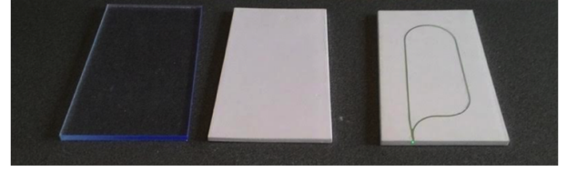
(a) Scintillator tile production for inner HCal
