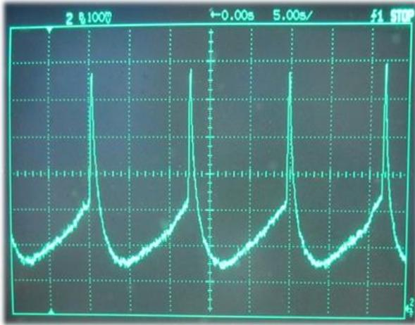
Fig. 6. The current waveform. The scaling for the y-axis is 100 mV = 6 A. The peaks are approximately 40 A. The time period between successive peaks is 12.3 Sec. Zero for current is the bottom horizontal line of the scale.
