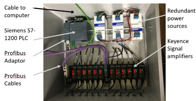
Fig. 7. The full assembly of the CMPS readout for the Detector Solenoid. Shown are the two Keyence DL-PD1 units with the six amplifiers for the IL-065 sensor heads (one Keyence IL-1000 master and five Keyence IL-1050 slaves). Redundant power supplies increase the operational functionality. A SIEMENS S7-1200 PLC with a CM2354-3 PROFIBUS master extension allows to read the sensor head data and compute the displacement.
