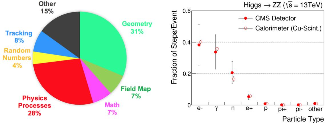
**Figure 1.** A standalone CMS detector simulation with  $H \rightarrow ZZ$  events from  $p\bar{p}$  collisions at LHC simulated with Geant4: (left) CPU allocation for linked objects, (right) the fraction of the average number of steps per event by the particle type.
