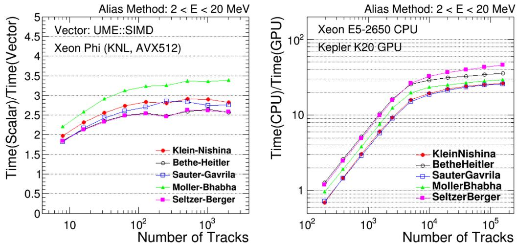
**Figure 3.** Performance results of simulating particles that undergo EM processes using the alias sampling method: (left) the relative speedup of the vector backend tested on Intel® Xeon Phi 7120 (Knight Landing) using UME::SIMD and the AVX512 instruction set with respect to the scalar code, (right) the ratio between the time taken by the cuda code on NVidia GPU (Tesla K20M) and by the scalar code on Intel Xeon (E5-2620).
