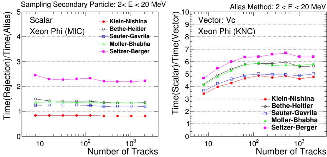
**Figure 2.** Performance results of simulating particles that undergo EM processes using the alias sampling method tested on Intel® Xeon Phi 5110P (Knight Corner): (left) the ratio between the CPU time taken by the alias method and by the Geant4 composition and rejection method (both scalar codes), (right) the relative speedup of the vector backend using Vc and the IMCI (MIC) instruction set with respect to the scalar.
