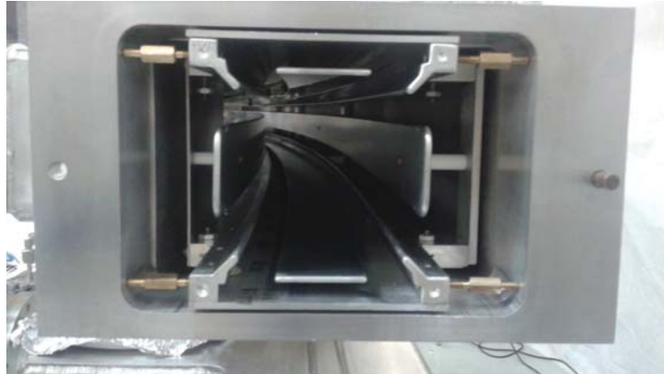
Figure 1. View of the cage with trolley rails and (most interior) four electrostatic quadrupole plates, from a vacuum chamber end flange.
