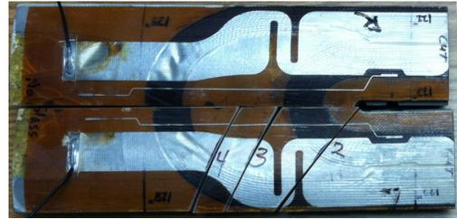
Fig. 4 HQ03 Coil Return End Autopsy
