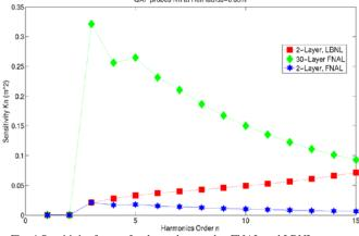
Fig. 4 Sensitivity factors for the probes used at FNAL and LBNL
