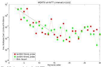
Fig. 5 Probe resolution for VMTF probe at room temperature.
