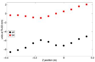
Fig. 11 Octupole harmonics as a function of axial position in magnet straight section
