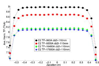
Fig. 9. Transfer function vs. axial position at various currents.
