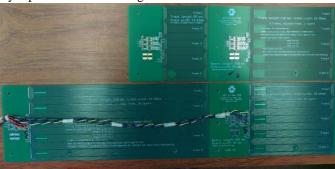
Fig. 1 Circuit board probes used for the measurements. Top: the 55 mm/110 mm 2-layer PCB; bottom: the 220 mm/110 mm 30-layer PCB.
