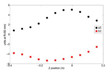
Fig. 10 Sextupole harmonics as a function of axial position in magnet straight section
