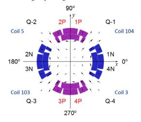
Fig. 7 Coordinate system definition for MQXFS1. Coils 3 and 5 were built by LARP and 103 and 104 by CERN. The 'P' and 'N' represent regions with positive and negative currents directed along +Z respectively.
