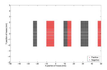
Fig. 2 Cross-section of the 30-layer printed circuit board used in the probe. The thickness is 4.5 mm and the width is about 80 mm (95 mm including the spare loop (not shown)).
