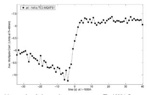
Fig. 14.  $a_4$  vs. time during a stair-step measurement. The 1000A flattop current is reached at t=0, and the dynamic effects decay within a few seconds.
