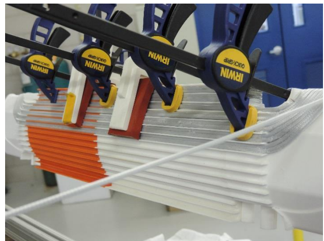
Fig. 4. Turn Placement on Inner Coil
