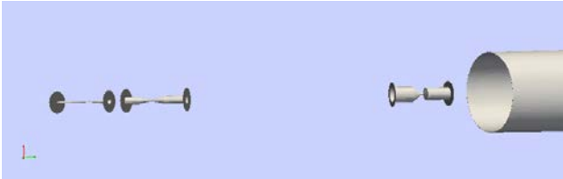
Figure 3: An optimized three-horn configuration. The proton beam comes from the left and the mesons produced at the target enter the decay pipe shown on the right.
