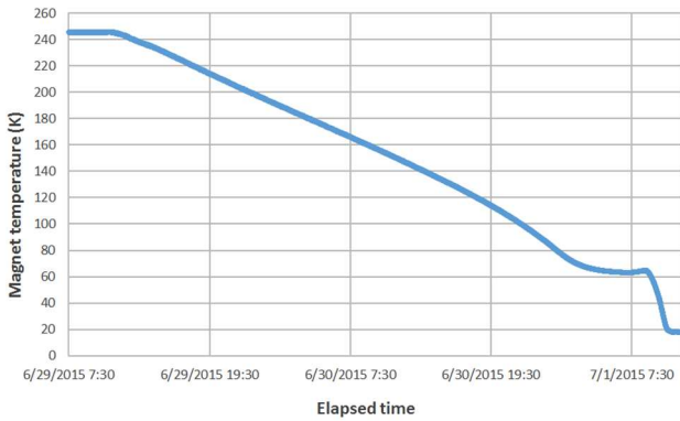
Fig. 6. The magnet temperature during cool-down.
