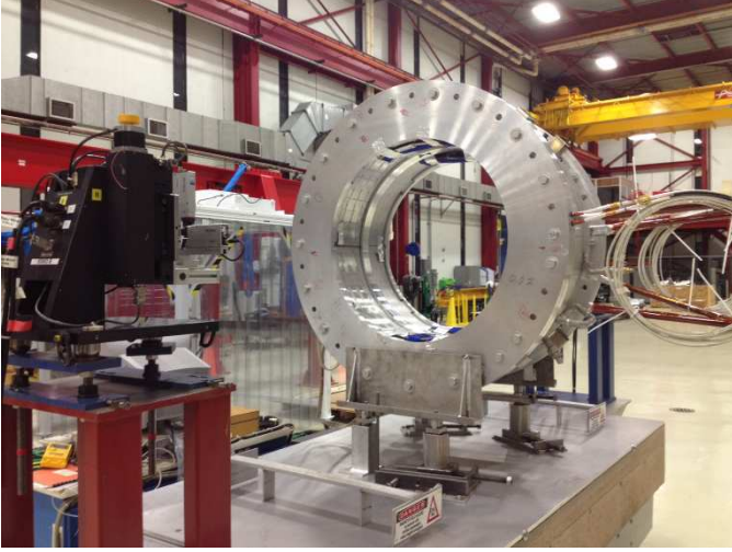
Fig. 3. The TS Prototype on the vibrating stretched-wire station.
