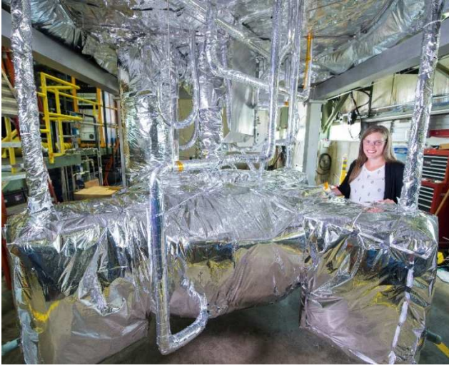
Fig. 5. The prototype with its custom thermal shield finalized and ready to be cold tested.
