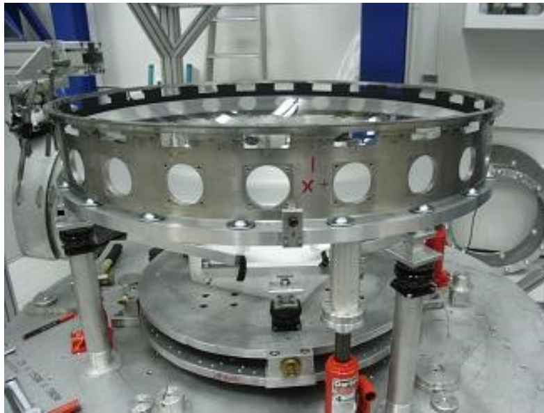
Fig. 14.— The C1 lens is partially installed in the C1 cell. The lens is supported from underneath on tip and tilt stages that are mounted on a rotary table. The cell is supported on jacks and its own tip/tilt system. This cell already has the thin steel ring mounted on its flexures.
