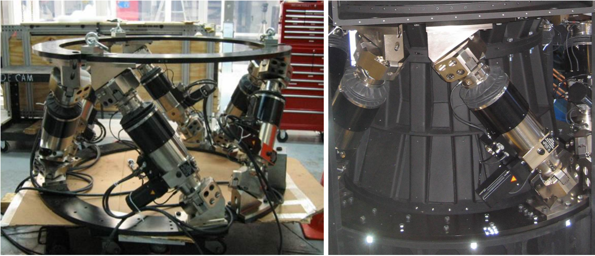
Fig. 42.— The assembled hexapod at CTIO. The picture on the left shows the six legs with the mobile flange on top and the fixed flange, which bolts to the cage, on the bottom. The picture on the right shows the hexapod, in the same orientation, with the fixed flange bolted to the cage (bottom) and the mobile flange to the body of the barrel. The flex joints are at both ends of each hexapod leg.
