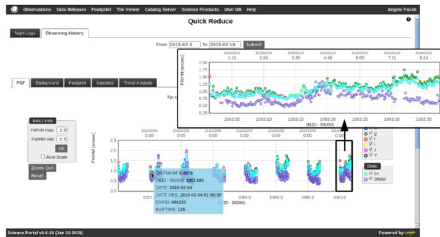
Fig. 54.— Quick Reduce results exported to the DES Science Portal at Fermilab. The plot shows the variation of the FWHM (arcsec) in the selected period of time. The points in the inset correspond to measurements on each exposure. The QR measurements are compared with the Image Health (cyan) and the DIMM seeing (violet) for reference.
