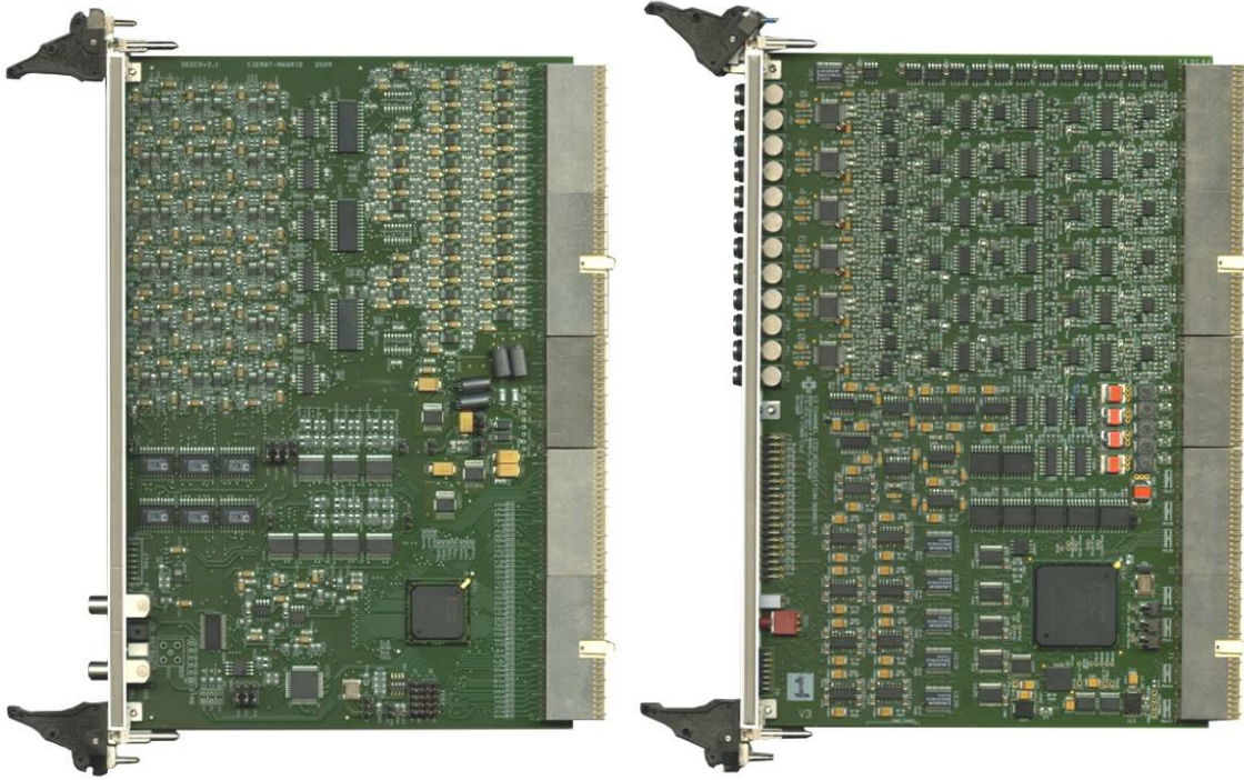
Fig. 34.— The DECam Clock Board main module (left) and 12-channel Acquisition Board (right) main module.
