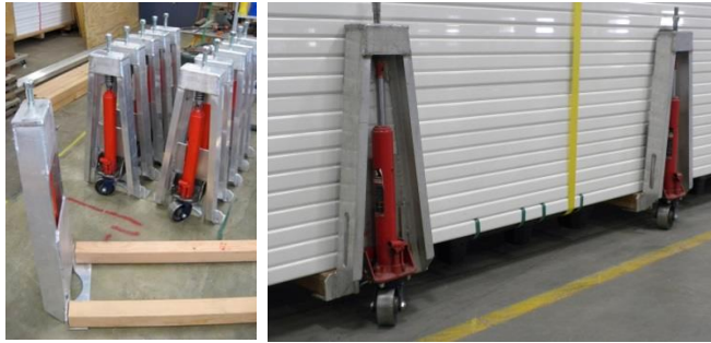
508 Figure 12: (a) Hydraulic caster jacks. (b) Jacks inserted under a stack of extrusions.
