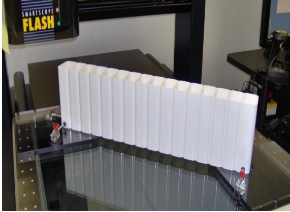
Figure 18: (a) A 15-cm extrusion placed on the scanning bed of the metrology machine. (b) The machine and operator console.
