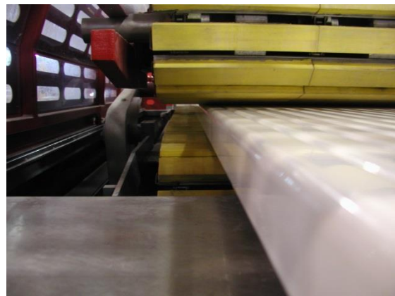
388 Figure 8: (a) Extrusion line. Shown in sequence are: the end of the extruding barrel (bottom of photo), the die, the sizing/cooling 389 section, and the puller (red). (b) Close-up photo of the puller showing treads pressing down on and pulling an extrusion.
