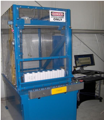
Figure 19: (a) The customized automated drop dart impact machine and (b) the resulting impacts on cells. Note the crack along a knit line in the upper cell.
