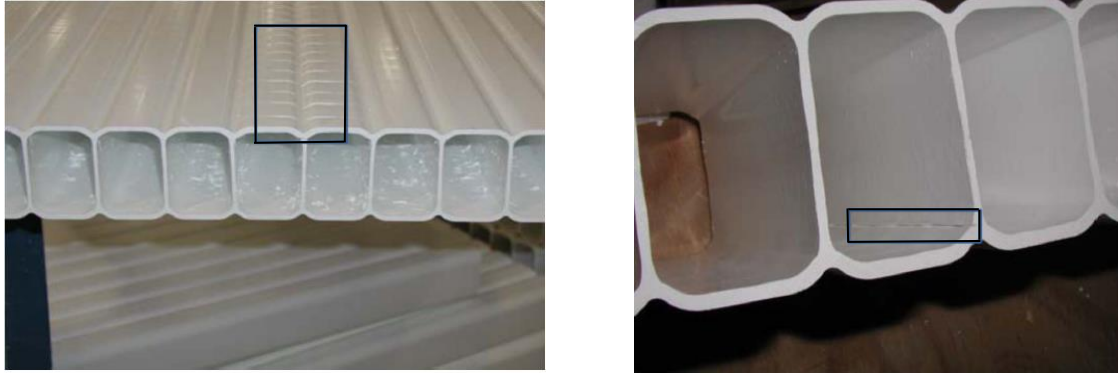
566 567 568 569 Figure 15: Example of extruding problems detected by visual inspection. Rectangular outlines added to the photos enclose (a) 570 chatter marks on the top surface (b) a poor knit in lower right corner. 571
