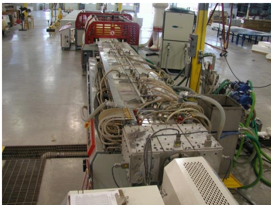
388 Figure 8: (a) Extrusion line. Shown in sequence are: the end of the extruding barrel (bottom of photo), the die, the sizing/cooling 389 section, and the puller (red). (b) Close-up photo of the puller showing treads pressing down on and pulling an extrusion.
