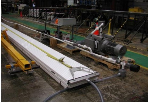
Figure 16: (a) The vacuum tester, with end-sealing manifold in place and the vacuum pump. (b) Close-up of the manifold, showing vacuum ports on odd-numbered cells. A second manifold on the other end evacuated the even-numbered cells.
