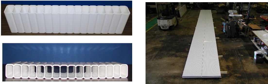
82 83 Figure 3: (a) Close-up photos of one 16-cell PVC extrusion, 15 cm long. (b) Two full-size 16-cell extrusions 15.5 m long placed 84 side-by-side form the basis for an extrusion module.
