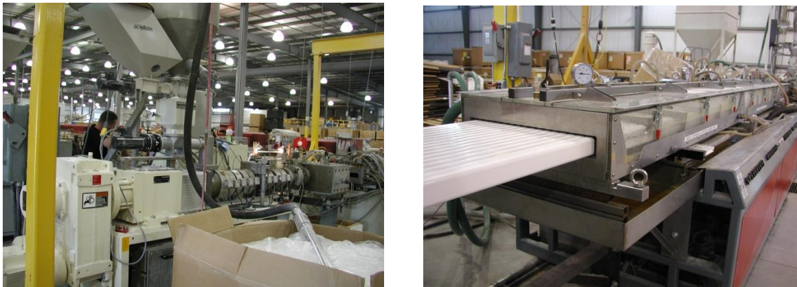
358 Figure 6: (a) N-27 powder is transported from a plastic-lined "gaylord" container into the extruder's hopper (top-center of the 359 photo). The extruding barrel and back-side of the NOvA die (right-center of photo) are also visible. (b) Rigid extrusion exits the 360 water cooling tanks and is about to enter the puller.
