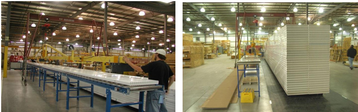
463 464 465 Figure 9: (a) The vacuum lifter, shown just above the extrusion, is supported by a movable gantry. An electronic weight scale is 466 attached just below the hoist, above the yellow frame. (b) The vacuum lifter is used to stack extrusions for transport to the module 467 assembly factory.
