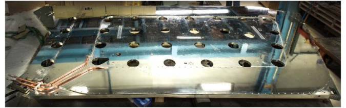
Fig. 10. Completed coil cold mass ready to ship.
