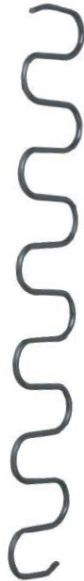
Figure 1: Example of a possible one-dimensional unit of which to build the bulk material. Individual spring-like elements can be interlaced and interconnected to construct a three-dimensional material. The individual elements will be resistant to the effects of thermal shock.
