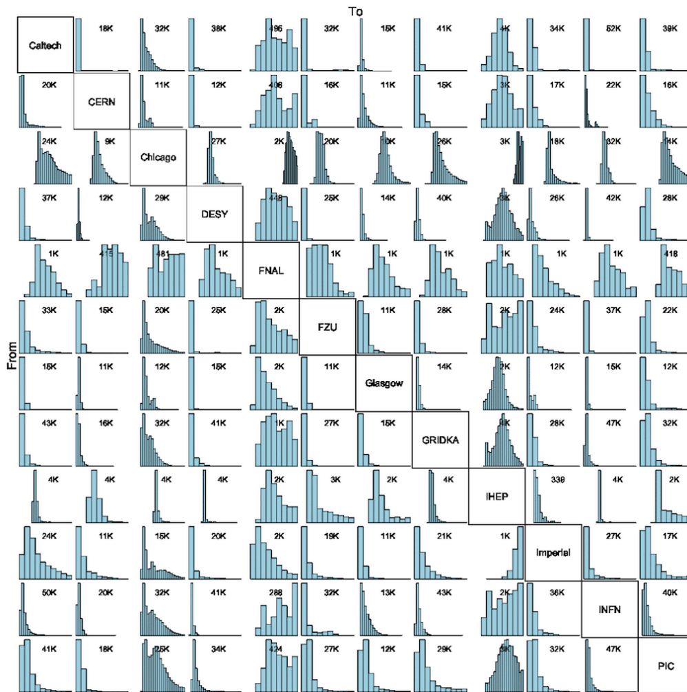
Figure 1. Transfer performance for the IPv6 testbed continuous transfers. A 1 GB file is transferred between each pair of sites, then deleted, then transferred again, continuously. The plots show the distribution of transfer duration times per site pair. The source site is named in the row, the destination site is named in the column. So the top-right plot shows transfers from Caltech to PIC, the bottom-left shows transfers from PIC to Caltech. The x-axis is in seconds, from 0 to 500 for each plot. The number inset in each plot shows the approximate number of transfers between that site pair in that direction.
